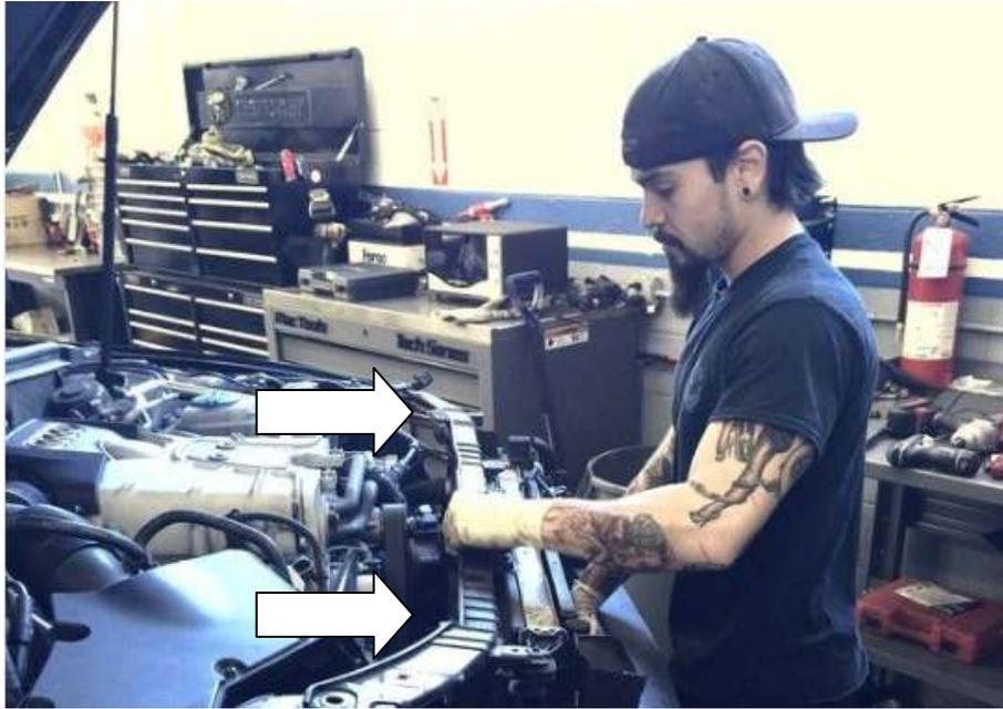
13. Use a 16mm socket and suitable ratchet to rotate the tensioner to release the tension on the belt and remove it.
