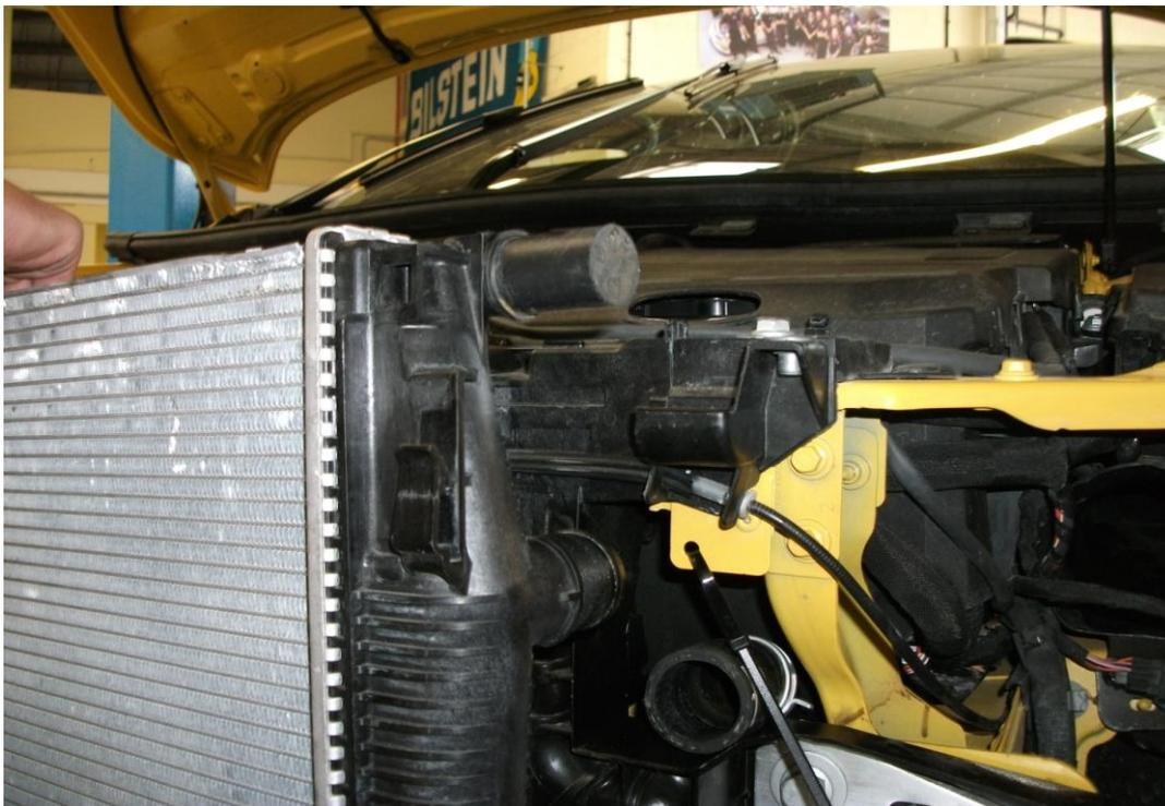
16. Pulling the bottom of the radiator out of the locating recess helps with ease of removal followed by lifting the radiator vertically to avoid damaging the condenser unit. Your radiator should now be removed.
