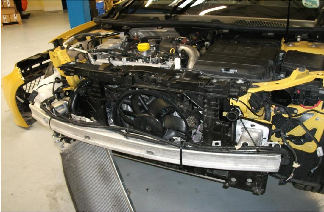
17. Now you can remove the four rubber bushes from the oem radiator and place onto the new alloy forge radiator.
