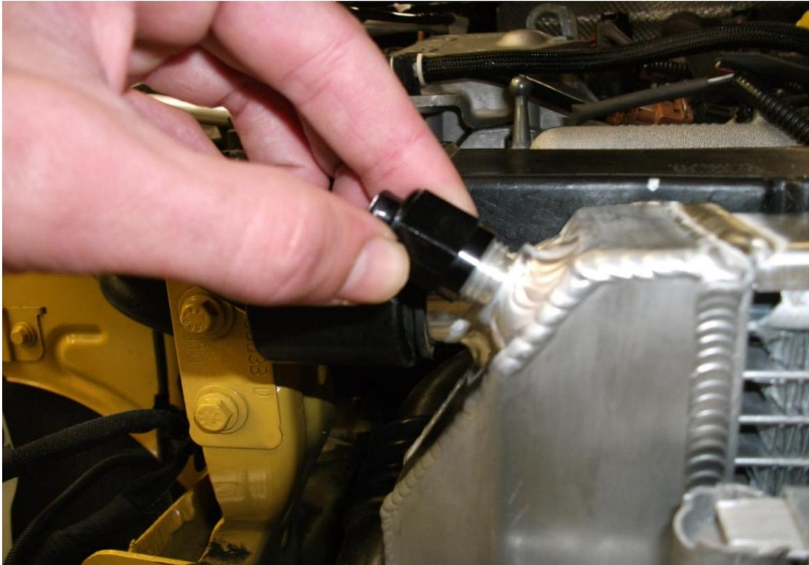
Also undo the bleed nipple located under the scuttle area near to the right hand side of turbo on a coolant hose that runs to the heater matrix .
