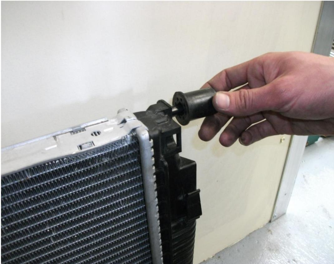
18. Once the rubber bushes are refitted to your forge radiator you can place it back into its original position, it makes it easier if you connect your inlet and outlet radiator hoses during the positioning of the radiator.
