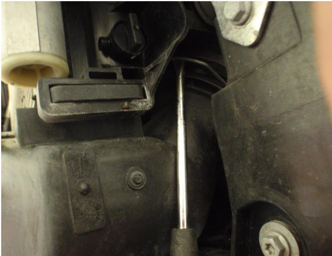
10. On the drivers side of the intercooler ,depress the clip holding the intercooler to the car with a flat bladed screwdriver.At the same time ,push the intercooler to the left (looking from the front of the car )to release from the bracket on the passenger side ,then pull down to release the passenger side connector.
