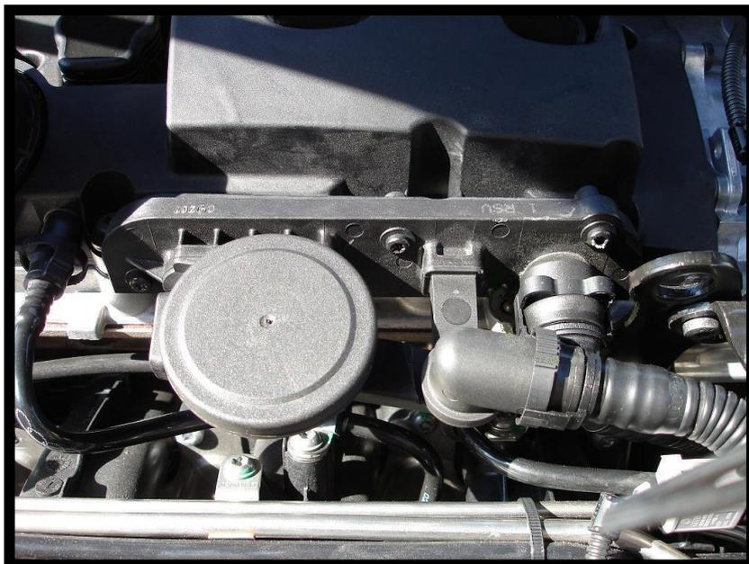
1. Unclip the breather pipes and undo the torx bolts, remove the PCV but keep to one side the rubber seal and torx bolts.
