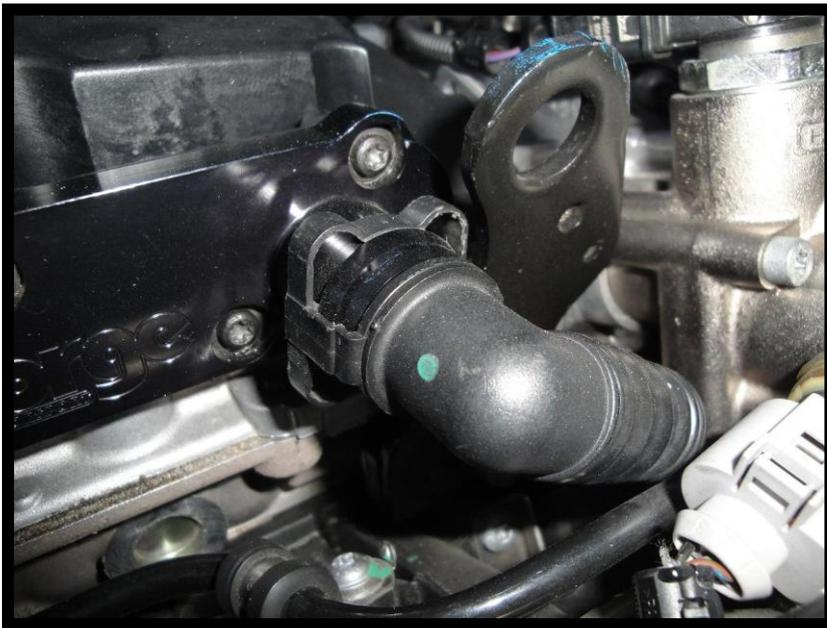
3. Attach the PCV delete with the OEM rubber seal and torx bolts and clip on the remaining breather pipe.
