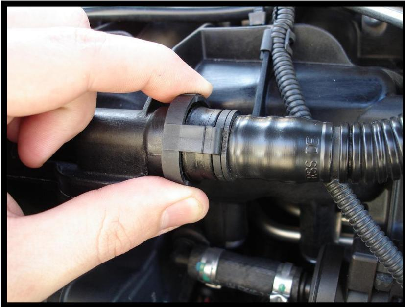
2. Unclip the breather pipe from the inlet manifold and remove.
