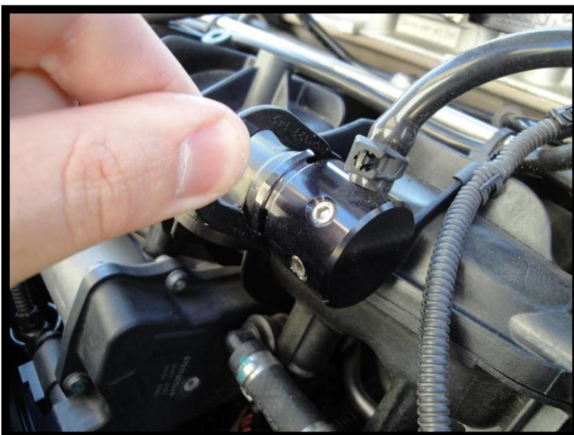
4. Attach the inlet manifold blanking cap with the plastic clip. Fully tighten the appropriate grub screws or boost gauge ports according to your needs. (We recommend applying a thread lock)
