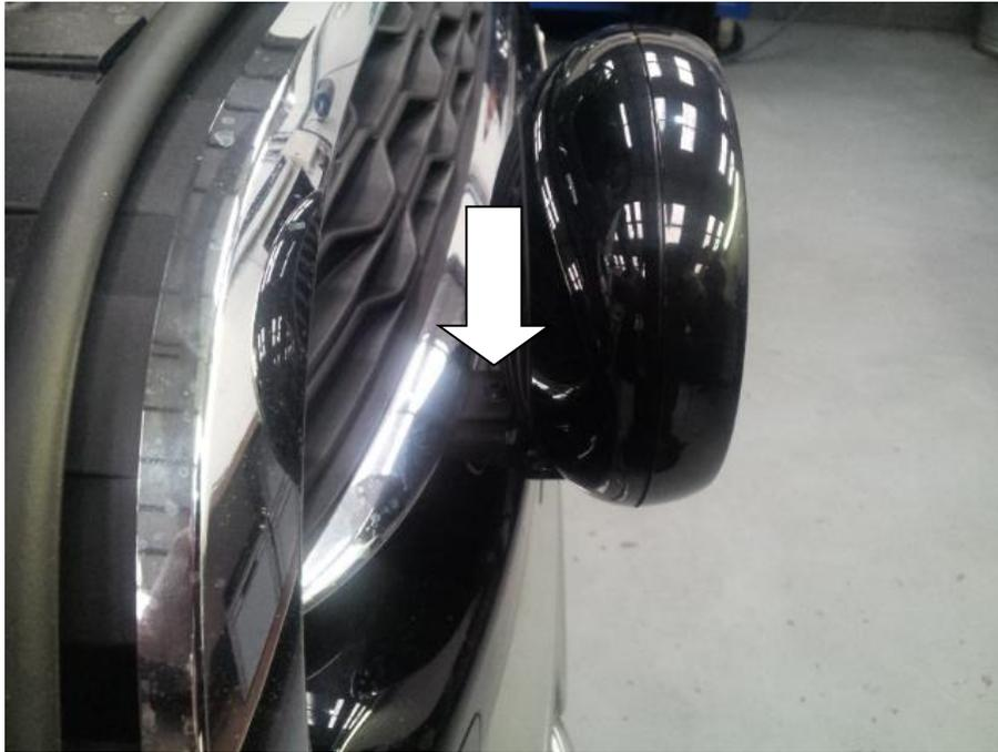
8. Undo the 3x T30 Bolts across the top of the bumper. You will require a second person to carefully pull the bumper forward and clear of the vehicle. Store in a safe place to prevent it from getting damaged while carrying out the rest of the installation.
