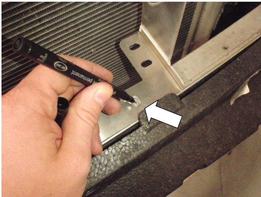
33. Using a 2mm drill bit, pilot drill a hole in the centre of the marked slots.
