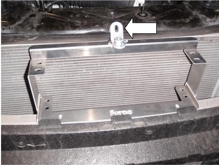
32. Using a scribe or marker pen mark the positions of the two holes in the base plate of the bracket on the crash bar.
