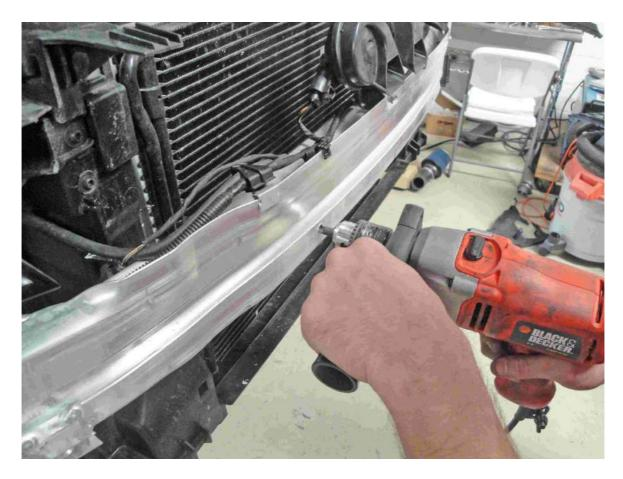
With the mounting holes drilled, position the Forge intercooler core in place again and secure it using the supplied hardware. Ensure that the core is tucked up flush against the underside of the bumper support to provide maximum clearance when refitting the bumper cover.
