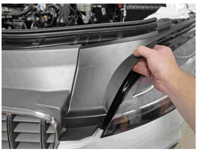
You can now remove the torx screws underneath each of these panels, as well as the screws located at the upper center portion of the grill next to the hood latch mechanism.
