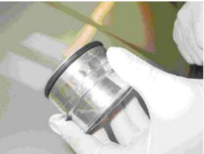
Fit the new aluminium hose coupling into it's respective fitting on the turbo outlet pipe running alongside the engine. Make sure the spring clip is affixed securely to prevent this coupling from being blown out of the pipe under boost.
