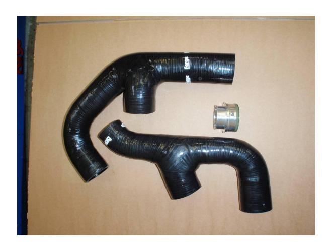
22.Offer up the driver's side hose first. Rotate the coupler in the hose until the tabs on the coupler line up with the tabs on the pipe and intercooler in the car. It's easiest to put the coupler in first, and then bend the hose to get the other end into the stock intercooler. Tighten the jubilees that hold the coupler to the hose, and then push the coupler in.
