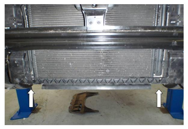
14.Offer up the intercooler to the front of the car, making sure the inlet/outlet pipes are behind the metal supports for the bumper that are welded to the front crash bar. The intercooler should naturally sit on the lower lip that you removed a section of in the last picture, and be about 5-10mm below the bottom of the crash bar.
