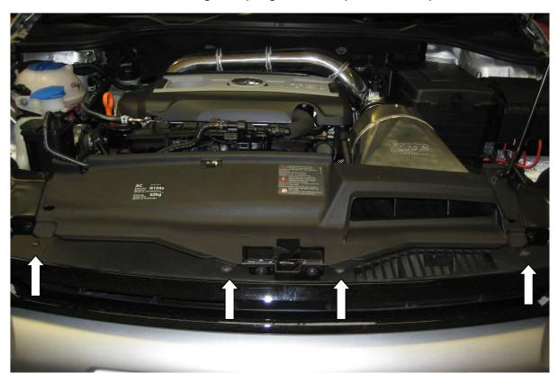
7. Pull back the edge of the bumper to release it from the plastic clips on the edge of the wing.
