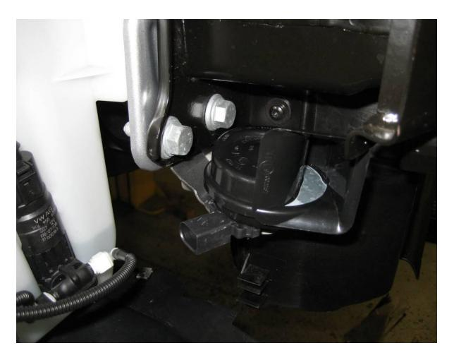
20.On the passenger side, remove the 12mm bolt that holds the horn bracket to the car and then using the right angled bracket provided, together with the M8x10 bolt, M8 washer and M8 nut, mount the bracket as shown below.
