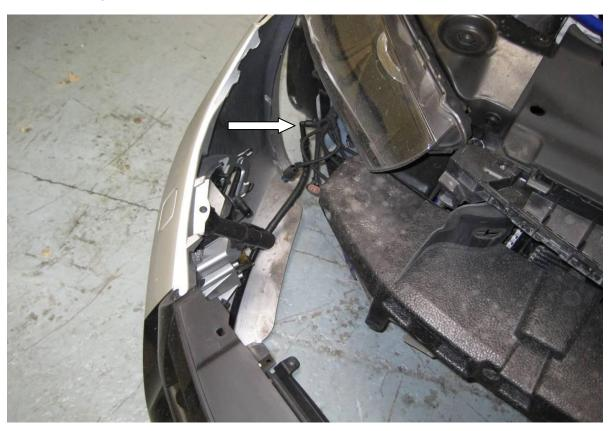
10.Place a bucket under the washer fluid reservoir and locate the bayonet fitting on the headlamp washer hose, then squeeze it to release and drain the fluid into the bucket. This will empty the whole washer reservoir (5 litres) so be sure you have something that can hold that amount. The bumper can be stored safely away for the time being.
