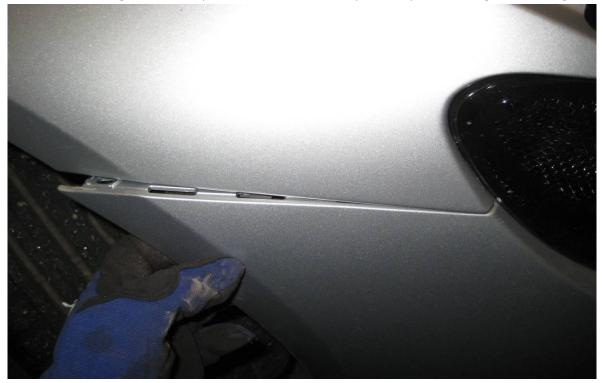
8. Get an assistant to support the bumper while you reach down behind and unclip the electrical connectors for the sidelights, fog lights and driving lights
