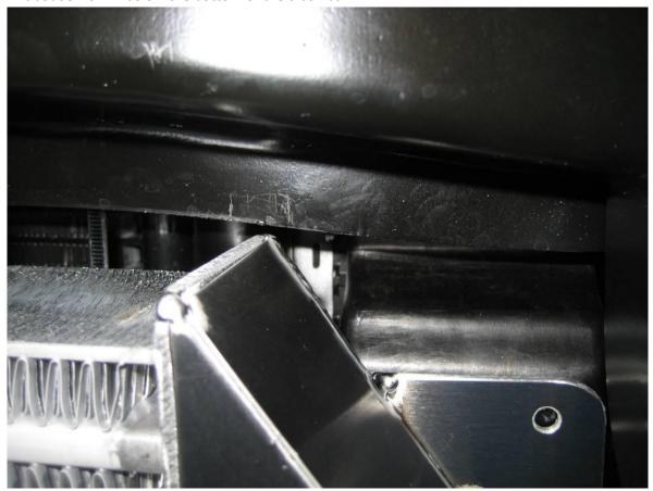
15. Mark the positions of the two screw holes at each end of the intercooler, then using a small 4mm drill, start a small hole, enough to get the self tapping screws started. DON'T DRILL MORE THAN 30mm DEEP. When you're finished, try starting the screw thread in the holes with the self tapping stainless steel screws provided.
