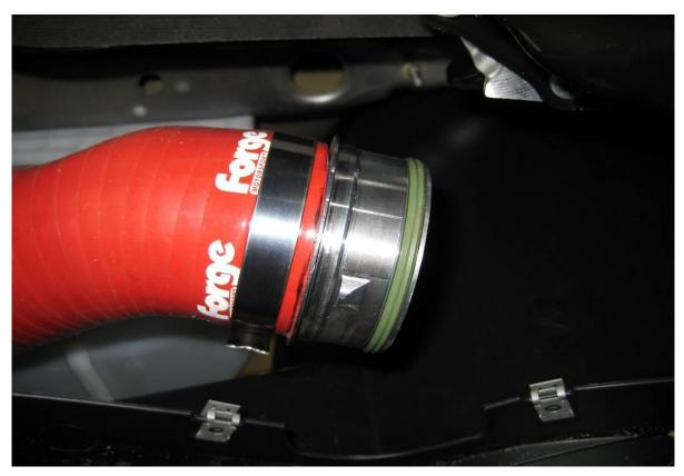
23.Place a jubilee clip on the front part of the hose, then connect it to the TWINtercooler and secure with a jubilee clip.
