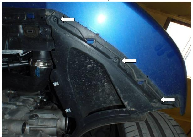
4. Undo the Three T25 screws down the inside edge of each wheel arch.
