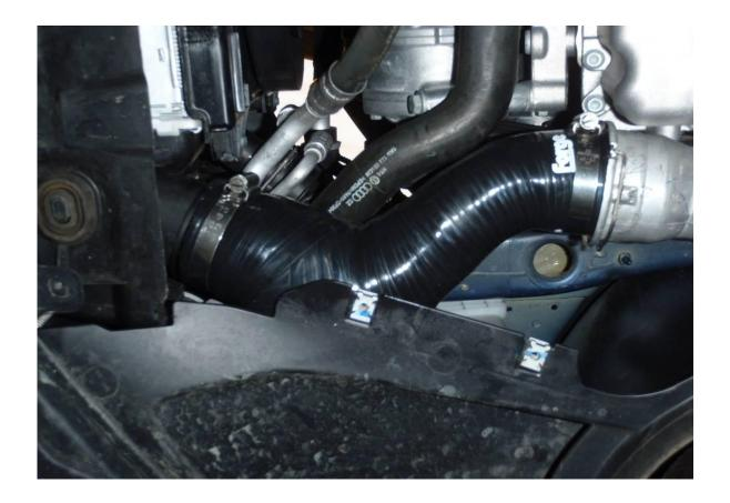
24. Repeat for the passenger side. Use a jubilee clip on the end to the intercooler and the end which goes to the throttle body. Tighten all the jubilee clips. Once all hoses are fitted you can now replace the transmission cooling duct.
