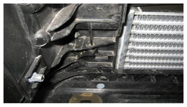
FOR REFERENCE – the screws aren't deeper than the reinforcement on the back of the Radiator cowl (picture from the back of the radiator cowl showing back of intercooler)
