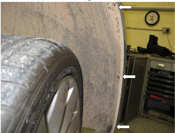
5. Undo the top T25 screw on the wheel arch liner. Pull back the top of the arch liner and undo the T25 screw holding the edge of the bumper up through the edge of the wing.
