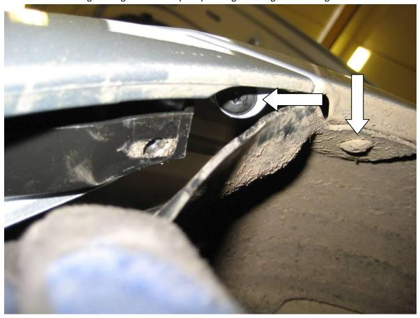
6. Undo the four T25 screws holding the top edge of the bumper to the slam panel.
