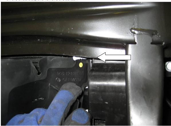
13.On the driver's side and passengers, cut out a small section of the lower lip in front of the radiator to assist in fitting the intercooler.
