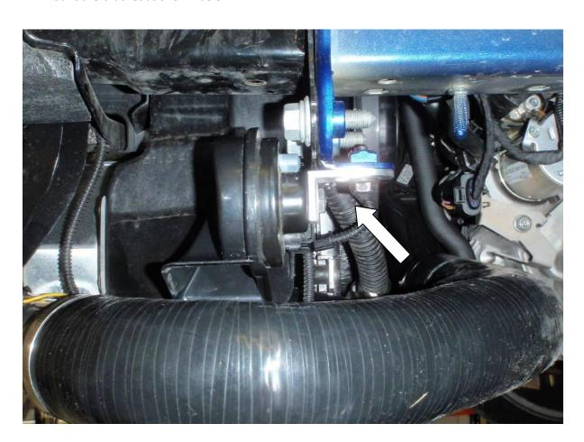
21.From the intercooler hoses you removed in step 8, remove the o-ring from the end and place into the Forge aluminium coupler. Try not to get any twists into the o-ring. Mount the coupler into the hose as shown below, with jubilee clips to suit. DON'T tighten the jubilee clips yet as the orientation of the coupler is important and it will need to be rotated.
