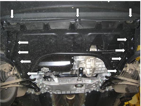
3. Undo three T25 torx screws of either side on the bumper
