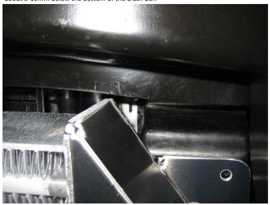
14. Mark the positions of the two screw holes at each end of the intercooler, then using a small 4mm drill, start a small hole, enough to get the self tapping screws started. DON'T DRILL MORE THAN 30mm DEEP. When you're finished, try starting the screw thread in the holes with the self tapping stainless steel screws provided.
