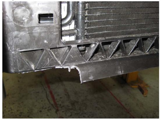
13. Offer up the intercooler to the front of the car, making sure the inlet/outlet pips are behind the metal supports for the bumper that are welded to the front crash bar. The intercooler should naturally sit on the lower lip that you removed a section of in the last picture, and be about 5-10mm below the bottom of the crash bar.
