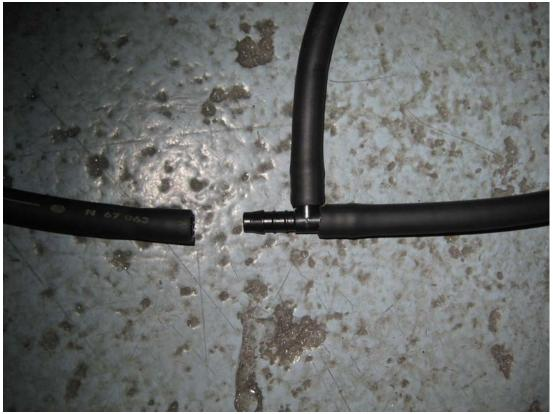
21. To facilitate fitting of the intercooler, we need to relocate the headlight washer tube. Using the supplied silicone hose, connect to the bayonet fitting and plug this in to the passenger washer. Secure it with one of the supplied cable ties. Route the hose as shown below, around the back of the foglight, and clip it in along the bottom of the bumper.
