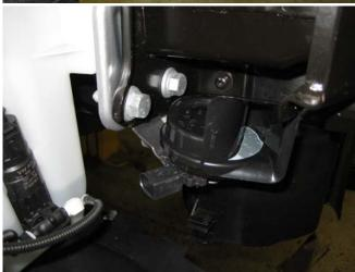
On the passenger side, remove the 12mm bolt that holds the horn bracket to the car and then using the right angled bracket provided, together with the M8x12 bolt, M8 washer and M8 nut, mount the bracket as shown below.
