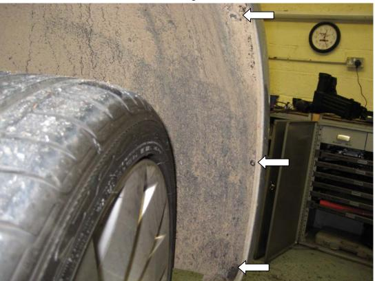
4. Pull back the top of the arch liner and undo the T25 screw holding the edge of the bumper up through the edge of the wing.
