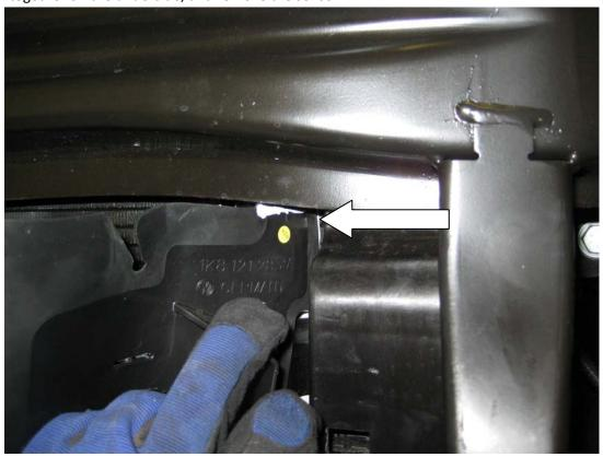
12.On the drivers side, cut out a small section of the lower lip in front of the radiator to assist in fitting the intercooler.
