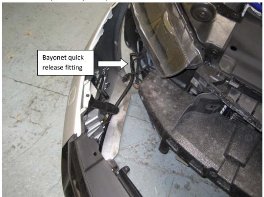
9. Place a bucket under the washer fluid reservoir and locate the bayonet fitting on the headlamp washer hose, then squeeze it to release and drain the fluid into the bucket. This will empty the whole washer reservoir (5 litres) so be sure you have something that can hold that amount. The bumper can be stored safely away for the time being.
