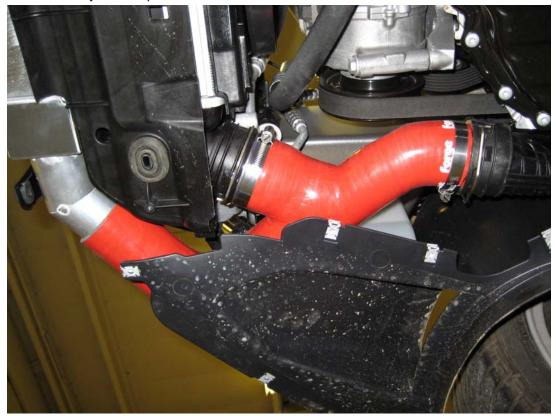
19. Repeat for the passenger side which is easier as there is only one aluminium coupler to contend with. Use a jubilee clip on the end to the intercooler and the end which goes to the throttle body. Tighten all the jubilee clips.
