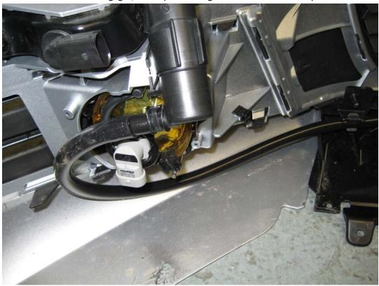
On the drivers side, connect the new silicon hose in to the tee piece, securing it with a cable tie, and route the hose as shown below.
