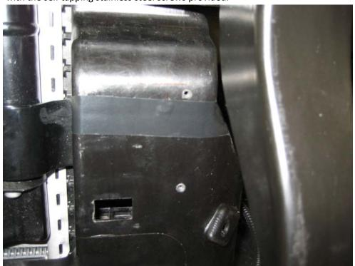
15. Offer the intercooler back up to the car, and make sure the holes line up, then screw the screws until they are all nearly tight, then screw each one in a little at a time to make sure the intercooler is flush against the radiator cowl. Don't worry about screwing in too far (see bottom picture). Push the air temp sensor onto its mounting until it clicks in place.
