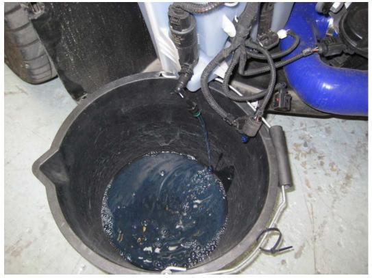
10. Working under the front of the car, remove both of the hoses that connect to the intercooler, by pushing a small screwdriver though the raised section of the c-clip and pulling to release the clip. The pipes can then be removed. Note that one connection is actually a jubilee clip which must be removed.
