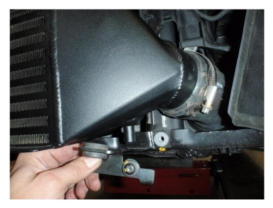
15. Now the intercooler is in the correct position, lift up the washer pipe out of the way.
