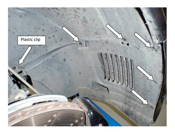
2. Undo the T25 torx screws under the front bumper and remove the arch liner.
