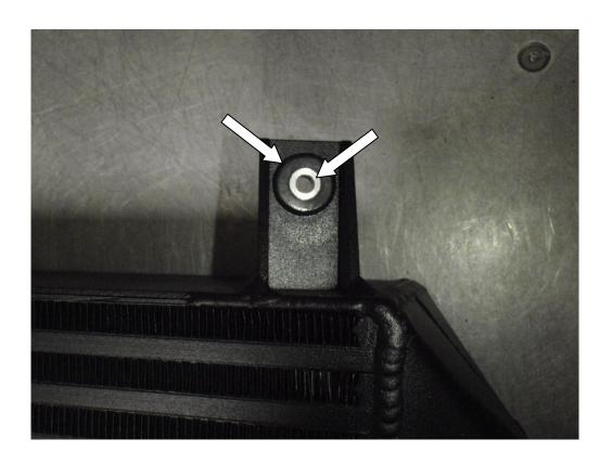
14. Place the uprated intercooler in position, attach the hoses and replace the existing intercooler brackets.
