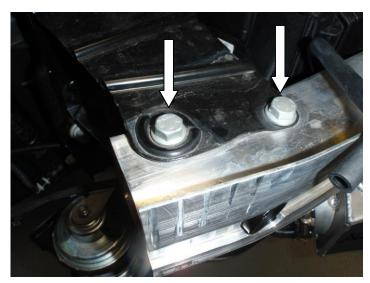
13. Insert the rubber grommets and aluminium sleeves into the intercooler, these are supplied in the kit.
