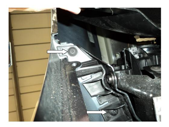
5. Remove the 13mm bolt from the back of the light - this is hard to see and reach but you can access from the inner arch.
