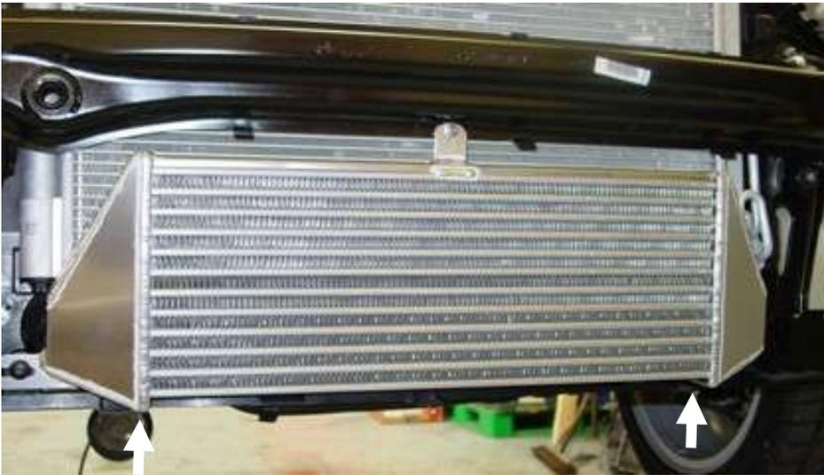
The Forge intercooler can now be installed into the hoses (do not tighten the clamps at this stage) and the two T25 Torx screws used to secure the intercooler brackets to the front panel. The rubber mountings of the original intercooler are not re-used. On the lower edge of the black plastic front panel there are slots that the intercooler end tanks will locate in (arrowed)
