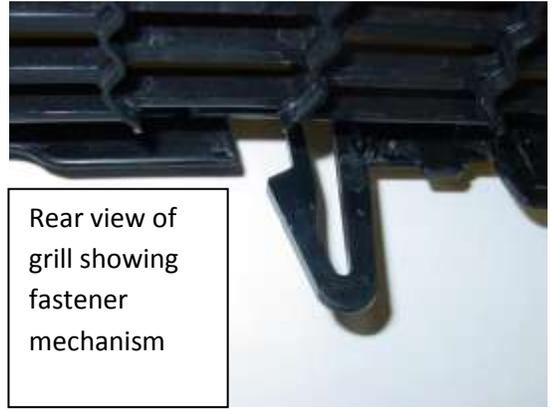
Rear view of grill showing fastener mechanism
