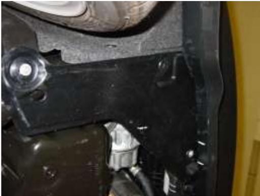
Depending on the vehicle origin it may be necessary to remove the plastic quadrants that fit between the wheel arch and the front of the vehicle, from underneath. These are secured by cross point screws that are rotated through 90 degrees to release.
