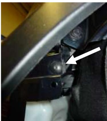
With the wheel arch trim loose at the front it is possible to access and remove the T25 Torx screw that secures the front panel. On both sides it is necessary to unplug the wires that go to the side and fog lights. (There is a tab on the plug that is squeezed to release the plug) and also disconnect the temperature sensor plug on the right hand side.
