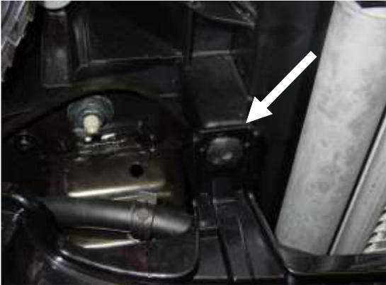
There are now two Torx T25 screws to remove. One on each side at the top of the bumper cover.
