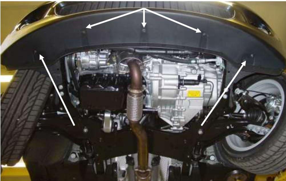
The underside of the bumper cover is secured by three of the push pin type fasteners and two T25 Torx screws (one each side).
