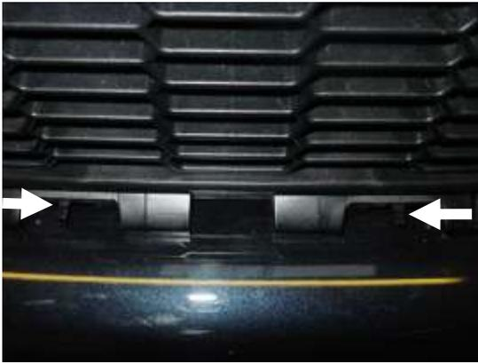
At the base edge of the grill there are four levers. When pushed towards the centre of the vehicle they allow the release of the grill from the bumper cover.
