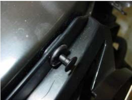
Firstly the vehicle will need to be secure and raised to allow the removal of the front wheels. The hood or bonnet of the vehicle should be opened. The grill needs to be removed. This is secured at the top edge by four plastic fasteners (push pins). The center pin of the fastener is prized out with the blade of a flat screw driver. This allows the fastener to be withdrawn from its locating hole.
