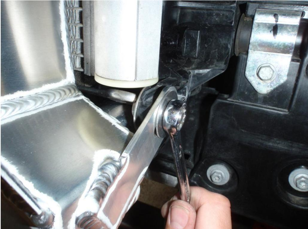
17. Bolt the horns loosely to the short bracket provided, then mount to the hole in the crash bar as shown below, using the M8x16 bolt, plain washer and nyloc nut. Orientate the bracket and horns as shown, getting the horns as close to the top of the intercooler to prevent them from hitting the underside of the bumper. Plug the horns back in to the loom.
