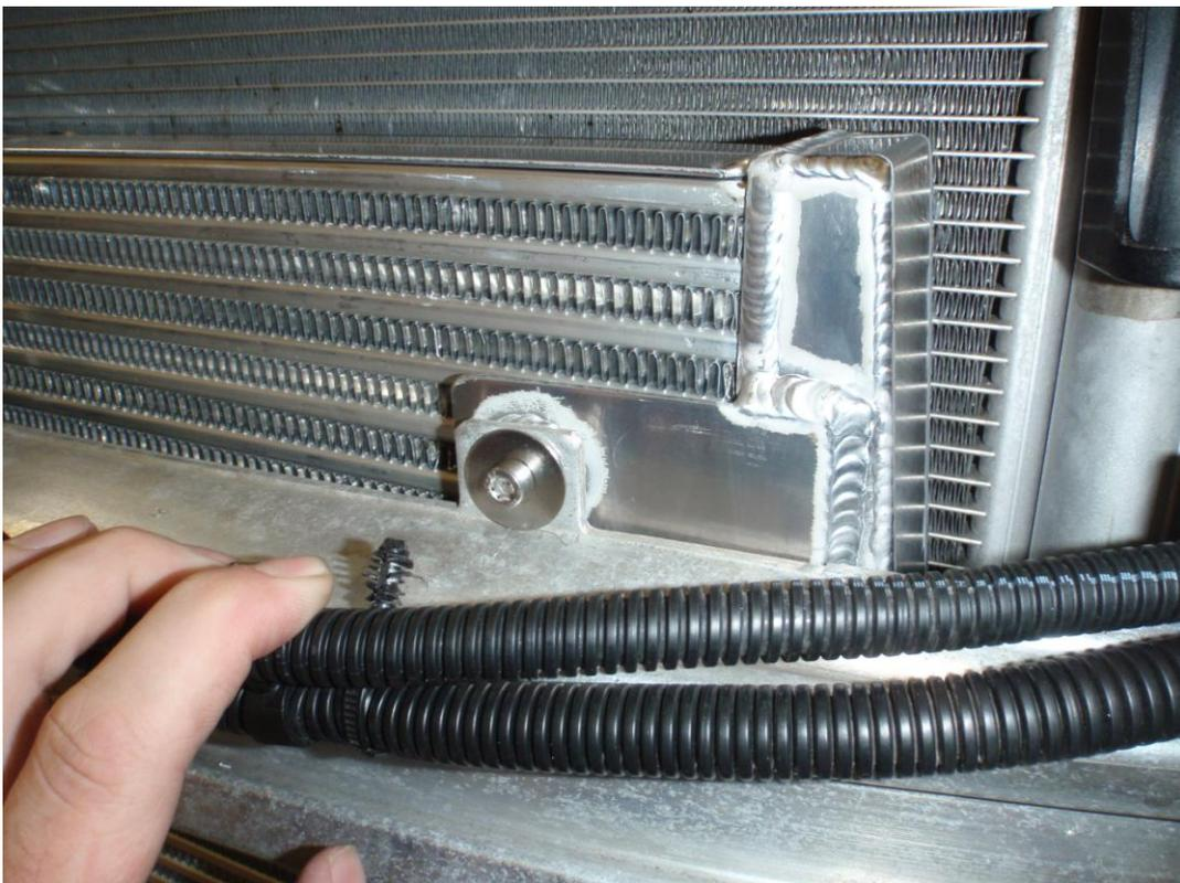
15. Push the passenger side into the hose first, until you hear a click signifying that the retaining wire clip is seated correctly in the recess of the connector. Make sure that the bracket shown below is on the OUTSIDE of the plastic attached to the car.
