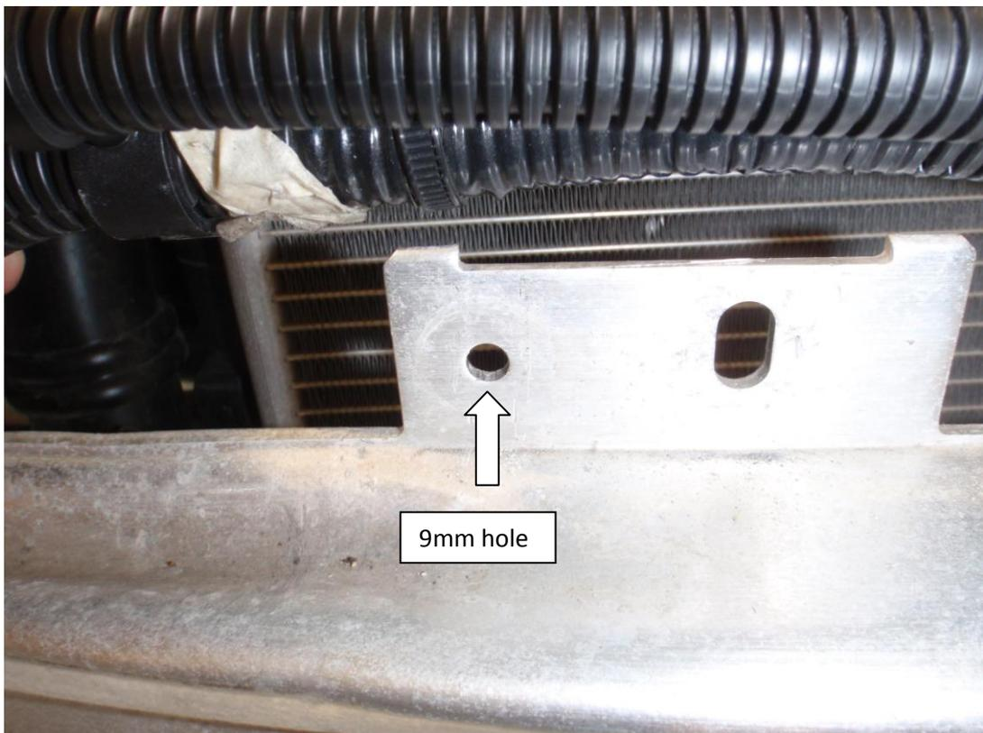
13. The crash bar needs to be loosened in order to fit the intercooler. Don't remove it fully as this will make it hard to mount the intercooler. There are three bolts holding the crash bar to the chassis **each end** (remove two and leave the last one in very loosely), and one 10mm bolt under the headlight that must be completely removed. The bolts on the chassis are unusually 5/8" head size so you will need an imperial socket set.
