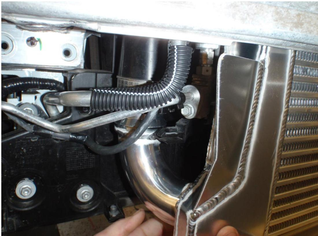
16. Refit and tighten the crash bar bolts removed in step 13. Tighten the two allen head bolts from step 14 full, and now use the provided M8x25 bolt, penny washers and nyloc nut to secure the lower bracket.
