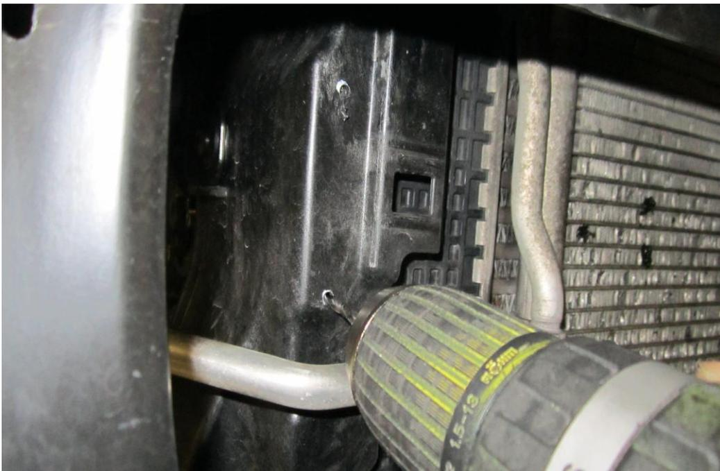
15. Once all four holes are drilled attach the twintercooler to the plastic cowling using the self tapping screws provided
