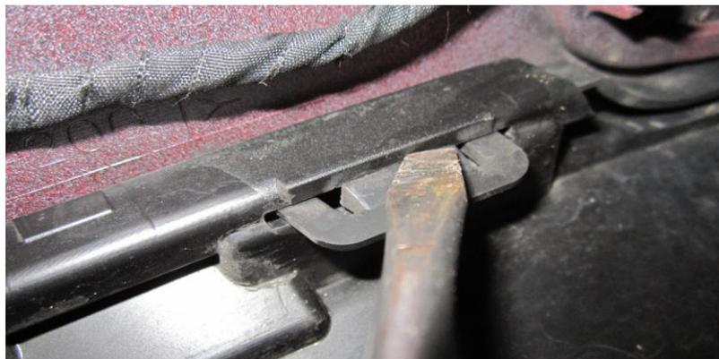
11. Remove the ducting either side of the condenser again using a flat bladed screwdriver .
