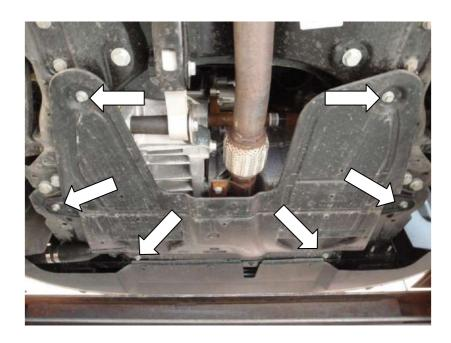
**4.** Undo the six 10mm bolts on the under tray using a 10mm socket and ratchet and remove.
