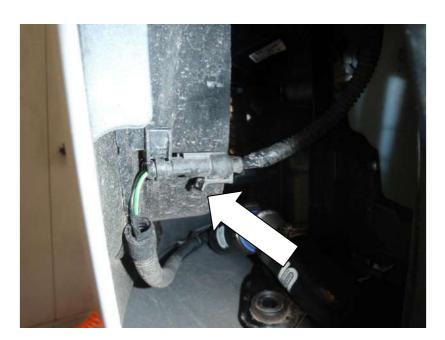
**2.** Additionally on the left hand side you will need to pull back the arch liner. You should see another connecter (see above). Pull the clip down and pull away to disconnect.
