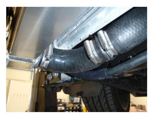
**27**. Push the long silicon hose onto the intercooler with a 55mm jubilee clip and do up in such a way that the bulky part of the clip is not on the bottom of the pipe because the intercooler sits slightly lower than stock. Place the 45mm hose joiner supplied in the open end of the hose and secure with a jubilee clip.
