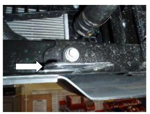
**14.** The brackets that were taken off with the metal pipe in steps 10 + 11 need to be replaced with the original bolts.
