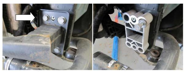
**20.** Hold your new forge motorsport intercooler up to the center of the middle crash bar and mark the boss locations with a paint marker.
