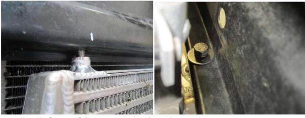
**24.** Tighten the fasteners fully using a 13mm ratchet and extension.
