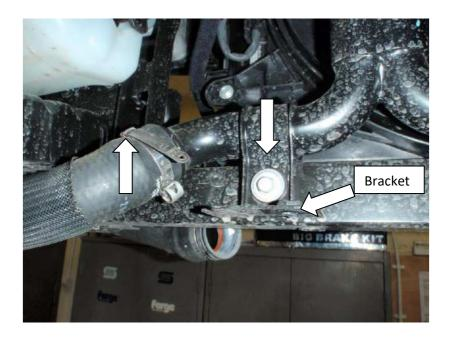
**10.**Looking at the back of the radiator you will see a large black pipe which is connected to a rubber hose from the passenger side intercooler, it has a 'use once' only clip this must be broken to remove. Undo the 10mm bolt shown, to remove the bracket keep to one side as this will need to be replaced once the pipe is removed.
