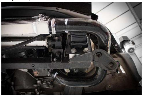
**28.** On the remaining silicon hose, loosely fit the 70 and 55mm jubilee clips. Push the large end of the hose onto the existing plastic pipe in the engine bay, and connect the other end to the joiner fitted in the last step. Tighten the jubilee clips. Now follow points 1-7 in reverse order and the installation is complete.
