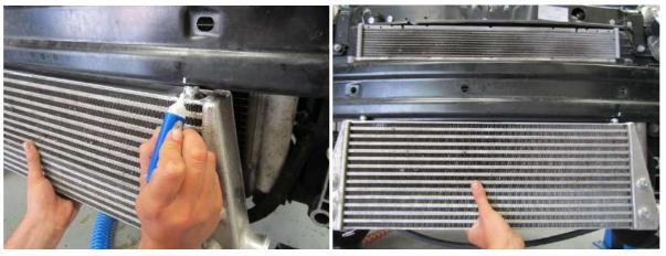
**21.** Using one of the M8 penny washers provided mark in the center of the washer inline with your previous marks on the underside of the crash bar as shown below.
