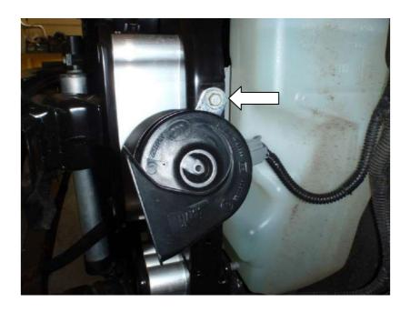
**17.** Using the bolt that was holding the intercooler move the horn up to the existing threaded hole and replace the bolt relocating the horn in a new position.
