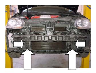
3/ Now remove the 2 horns and brackets. Use the right hand bracket and mount the left horn with this, you should be able to use the same body mounting point but this will raise the horn position in order to make space for the intercooler pies at a later stage. Use the mounting bracket supplied to mount the right horn as pictured below.
