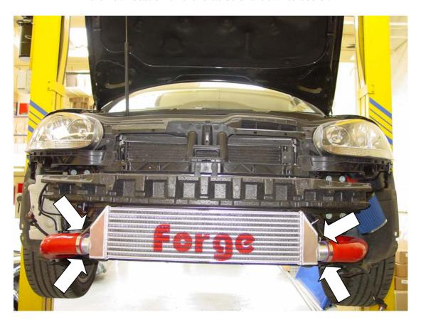
6/ Now fit the new 3 way hoses to each side of the intercooler and the new twintercooler using the hose clips supplied. Routing should be as pictured below. Tighten all hose clips securely once the hoses are fully positioned.
