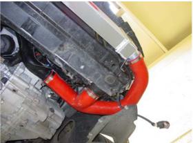
6/ The front bumper will now require the 2 fog light panels removing; these are fixed by a single pozidrive screw. Carefully refit the front bumper cover but do not force this on. Note if any areas around the fog light fixings are contacting with the new twintercooler piping. If they are then mark the area and then remove the front bumper and trim these areas with a sharp knife, you may have to cut as per the pictures below however some cars may require no trimming at all in this area.
