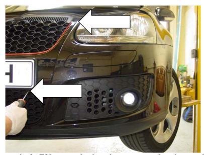
Now remove the 2x T30 screws that have been uncovered on the top edge of the bumper cover. Remove the 5x T20 Screws down each front wheelarch liner leading edge. Remove the 8x T20 screws from the lower edge of the front bumper. Disconnect both front fog light connections. The complete bumper cover is now ready to be removed by sliding the upper side fixings forward, remove the full bumper cover from the vehicle.
