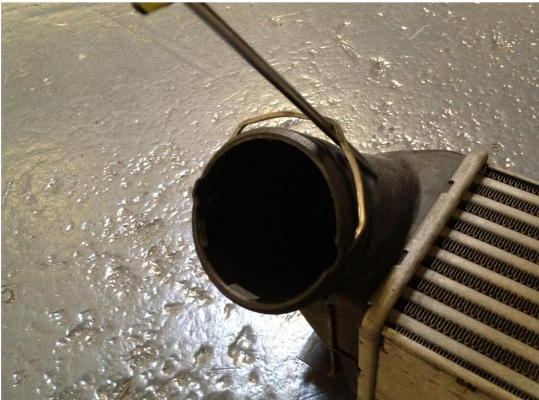
8. Push the Forge intercooler up into the space in the bumper – it may be easier to pull the arch liners out from the bumper to give you more room, and guide the intercooler hoses in at the same time. Once in place, do up the screws you removed in step 5, making sure that the fan assembly is clipped on the back of the intercooler as you do up the screws.
