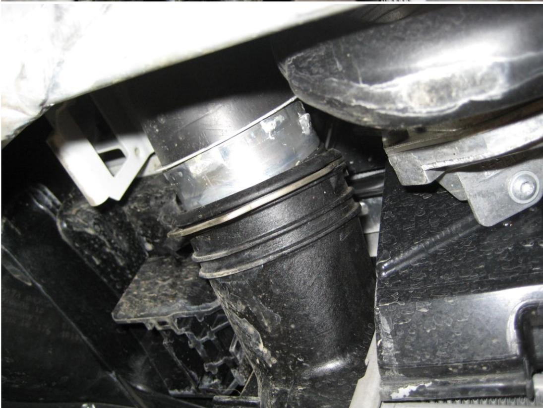
4. Rotate the two clips on the underside of the intercooler to the 'unlocked' position, and remove the plastic piece under the intercooler that they were securing.
