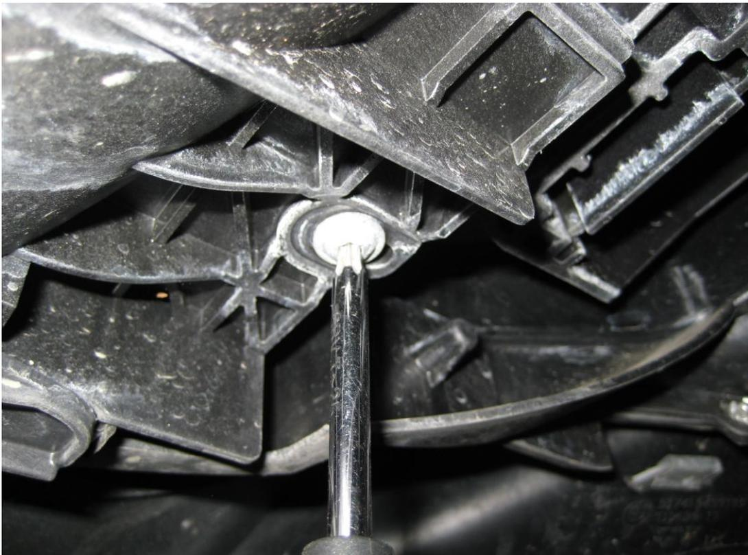
6. Remove the intercooler from the car with care. On the 335 it's necessary to bend back the lower edge of the bumper to facilitate removal, and moving the lower edges of the arch liners out from inside the bumper will help. Take care that the clips on the back of the intercooler release from the fan shroud.
