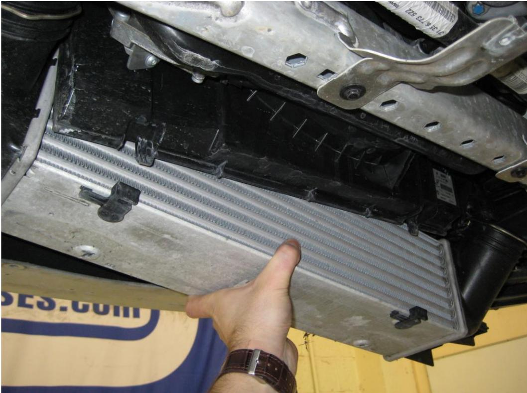
7. With the intercooler removed from the car, prise the hose retaining clips off using a screwdriver, and place them on the new Forge intercooler.
