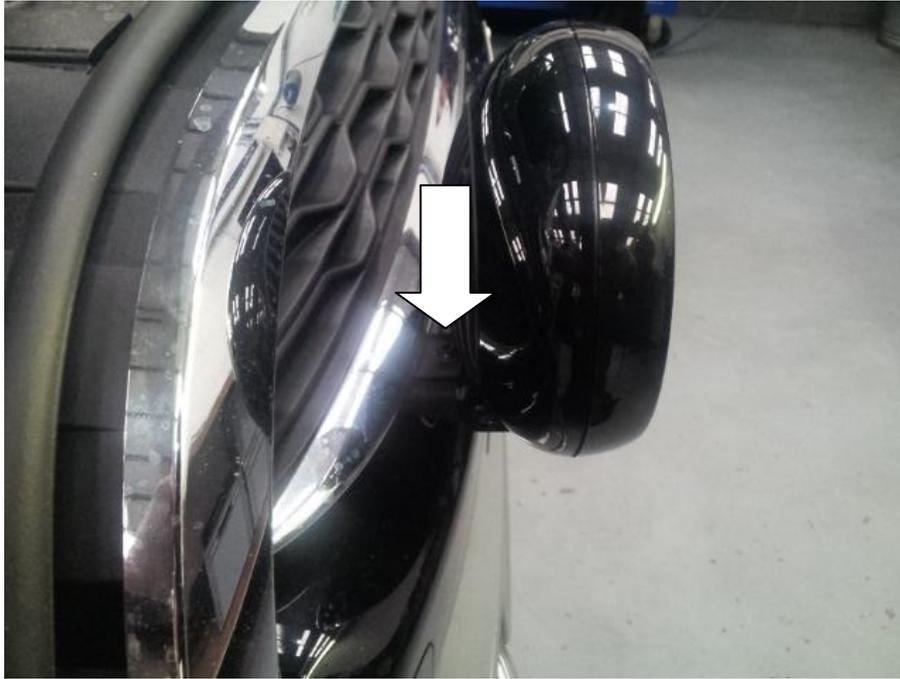
8. Undo the 3x T30 Bolts across the top of the bumper. You will require a second person to carefully pull the bumper forward and clear of the vehicle. Store in a safe place to prevent it becoming damaged while carrying out the rest of the installation.
