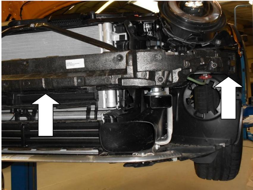
10. If fitted to your vehicle, unclip the wiring and using a T30 Torx driver undo the 2x bolts and remove the active air ducting.
