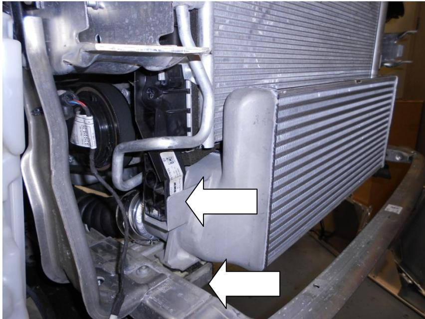
29. Using the 2x M8x16mm Allen cap bolts and 2x 8mm Penny washers supplied secure the intercooler to the bottom mounts.
