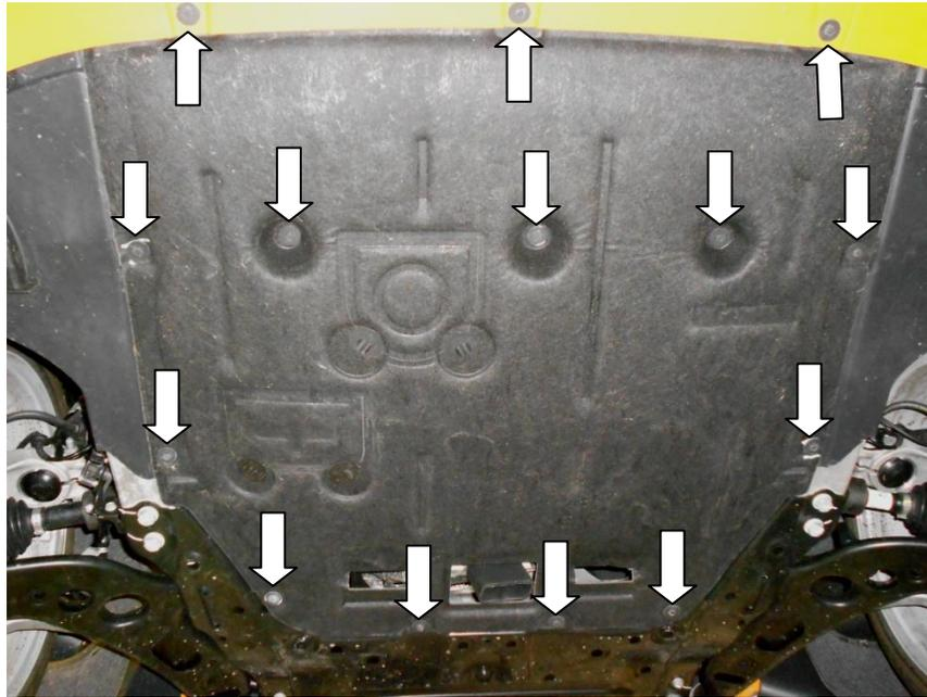
3. Using an 8mm socket and suitable ratchet undo 2x bolts in front of each wheel.
