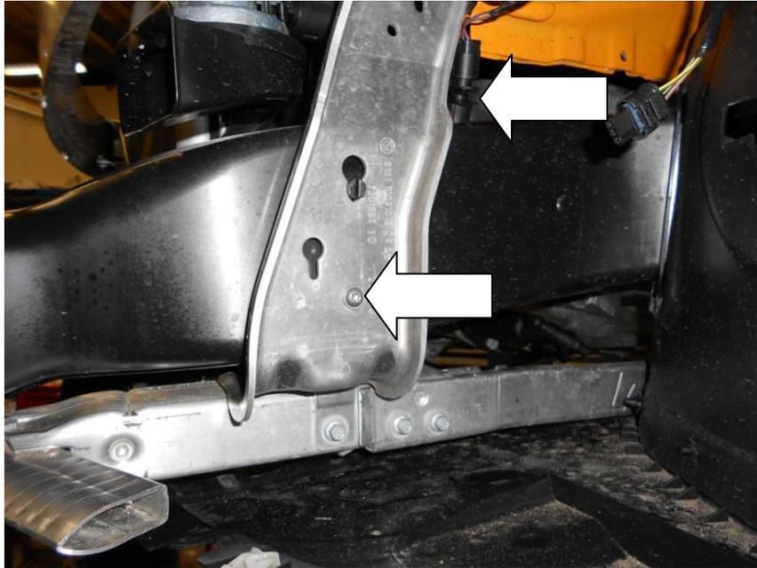
17. To access the bolt for the other duct you need to move the washer fluid reservoir. Using a T30 Torx undo the 2x bolts lift the reservoir upward to release it from its bottom mounts. To support the reservoir cable-tie it to the bracket above.
