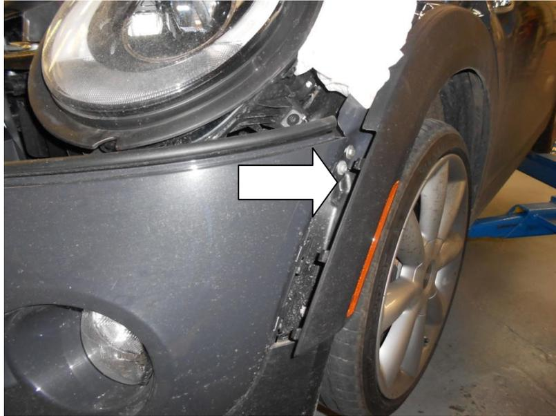
7. If your vehicle is fitted with Spot lights use a 3mm Allen key to loosen the horizontal bolt. Tilt the light forward using a 2mm Allen key undo the bolt and remove the headlight. Note the next part requires 2 people as the wiring connectors can only be undone once the bumper has been removed from the vehicle.
