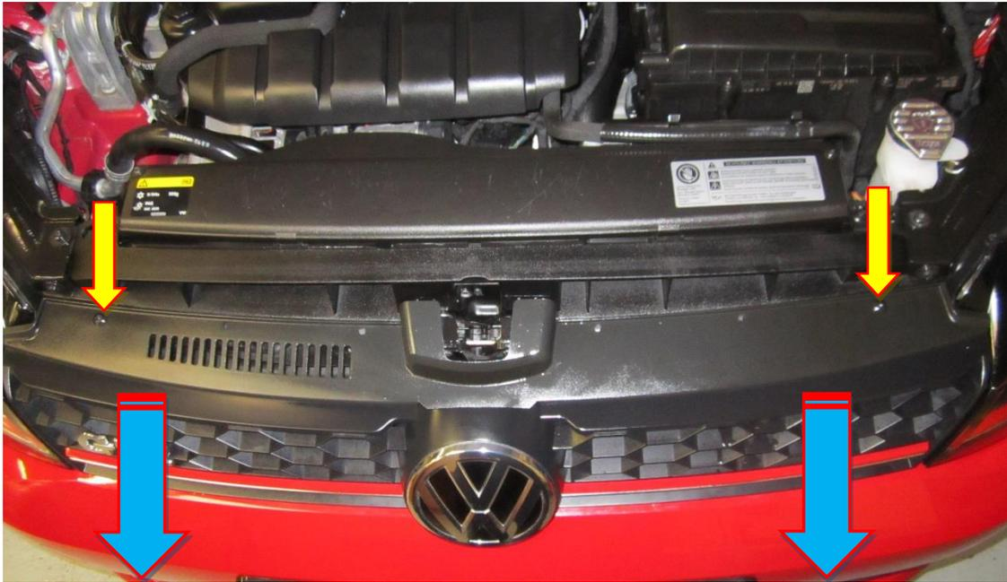
3. Using a T25 Torx and drive remove the x2 M5 fasteners that hold on the airbox duct and use a hose clamp removal tool to loosen the inlet hose from the air box.
