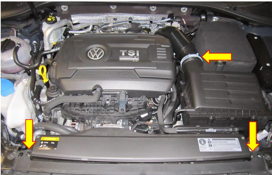
4. Unclip the coolant hose from the front of the airbox lid. Disconnect the vacuum hose attached to the front left of the airbox.
