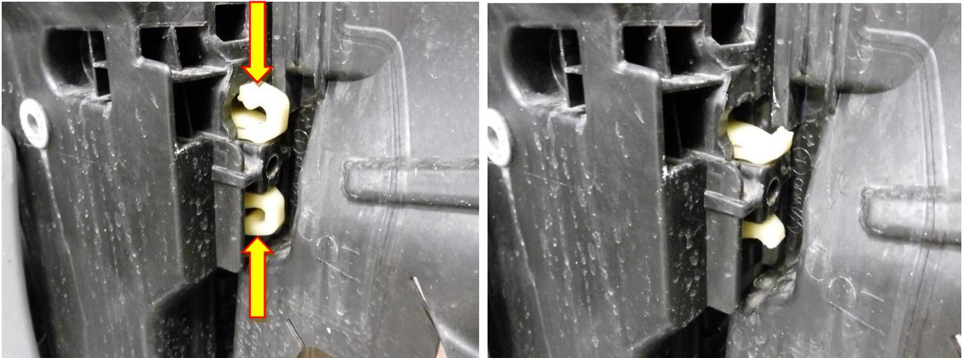
29. Using a flat blade screwdriver or trim tool, push both retaining clips down to separate the radiator from the intercooler. Once parted lift the radiator upwards from the intercooler to completely remove the radiator from the intercooler.
