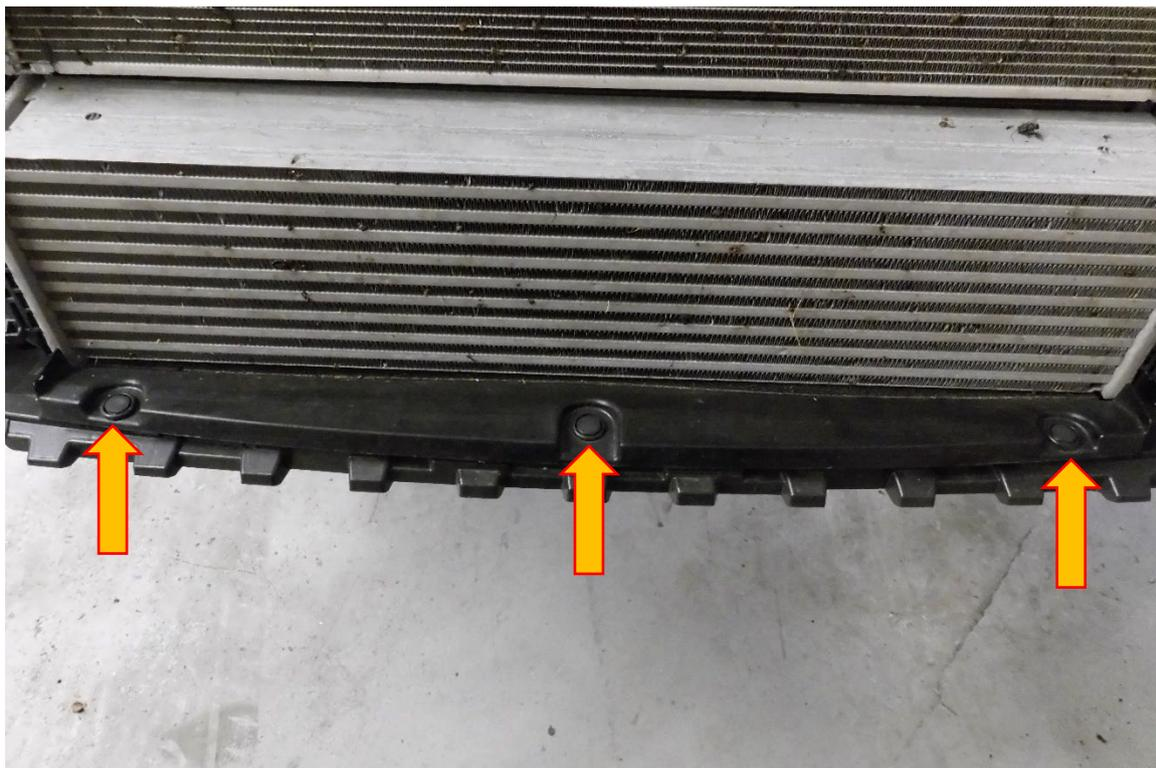
16. Using a 10mm socket and ratchet remove the M6 fasteners attaching the plastic panel below the intercooler. The intercooler will now come away from the vehicle.
