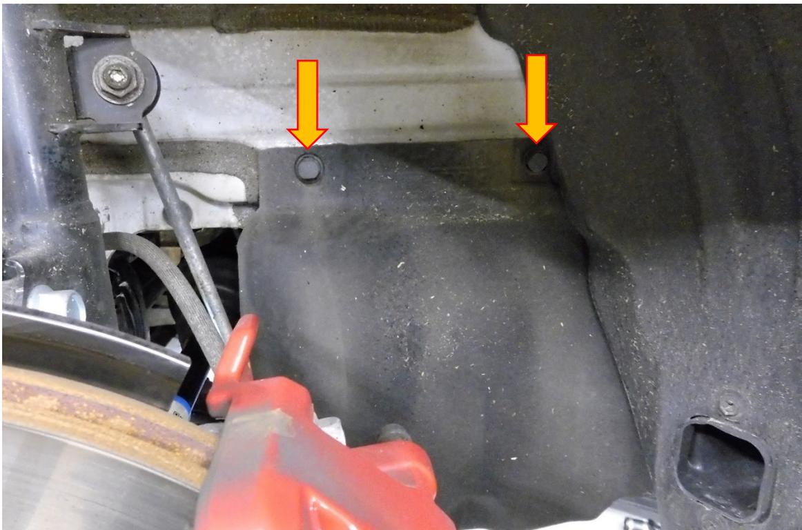
21. Using a 12mm socket and ratchet remove the 2X fasteners attaching the offside boost pipe to the chassis. Loosen the hose clamp attaching the turbo end of the boost pipe.
