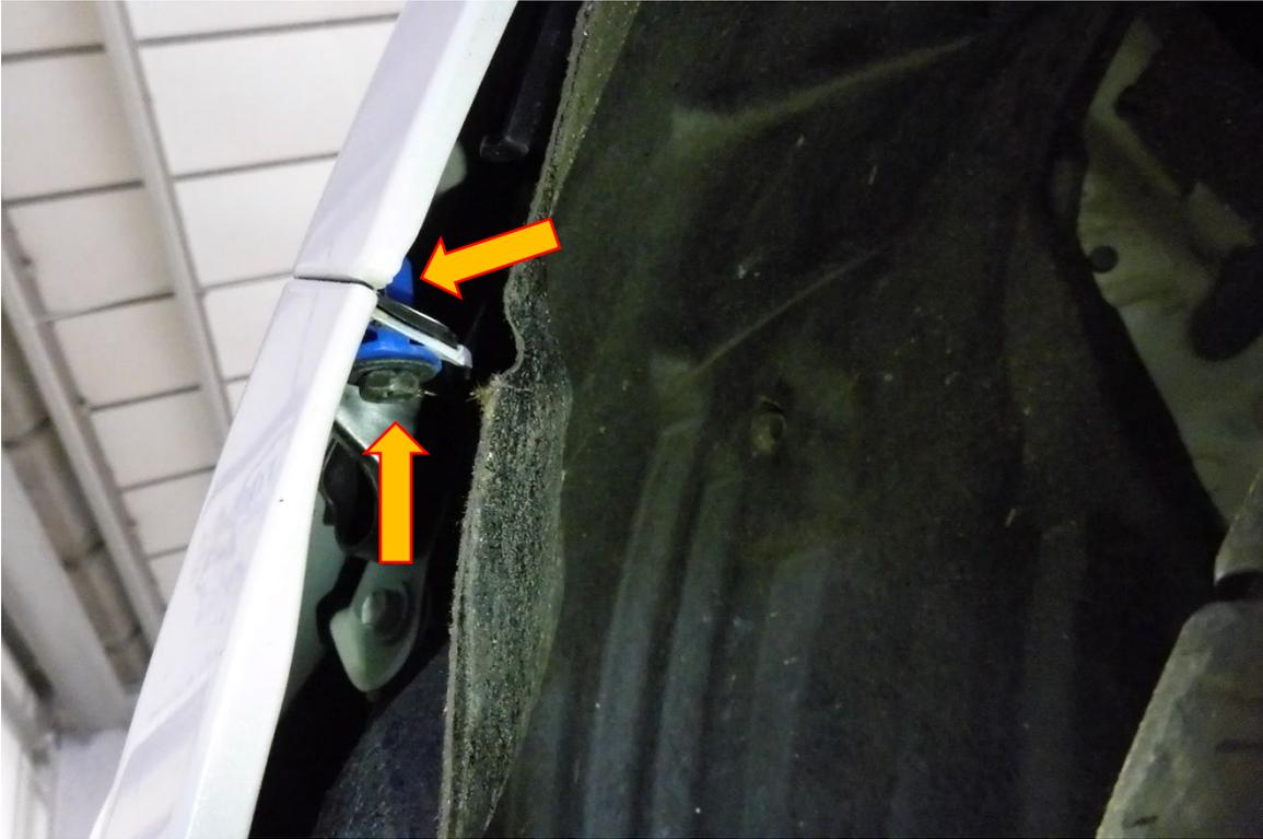
8. Using a plastic trim tool open up the retaining clips to allow the edge of the bumper to come away from the wing. Use some masking tape to avoid marking the paint work. When both sides are free from the wings carefully rest the bumper and unplug both fog light wiring looms.
