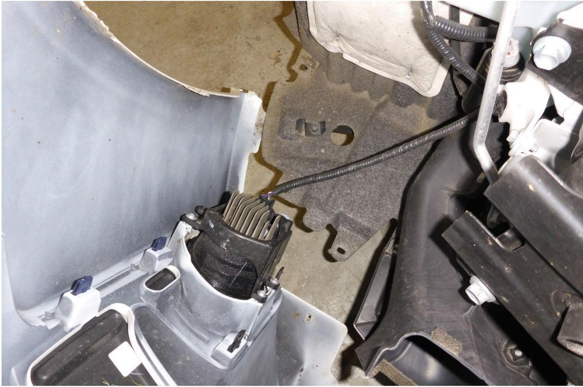
9. Removing the crash bar. Using a 17mm socket and ratchet there are 8 X M10 fasteners that need to be removed, 4 X each side. Using a 10mm socket and ratchet remove 2 X M6 retaining nuts, 1 each side. Unclip the horn wiring loom which is attached to the top of the crash bar.
