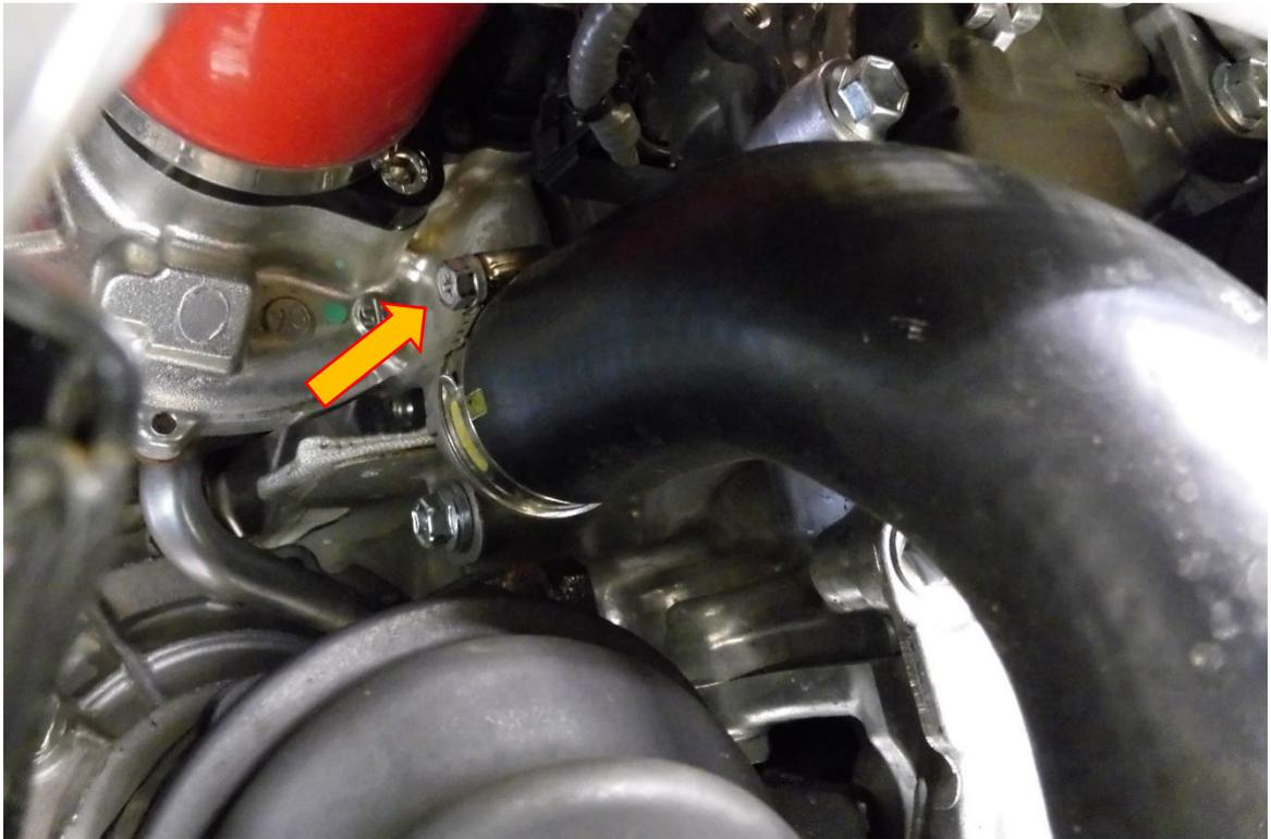
22. Fit the small end of hose #2043 to the turbo, use a 7mm socket and ratchet and the supplied 32-50 hose clamp from the kit to secure the hose to the turbo.
