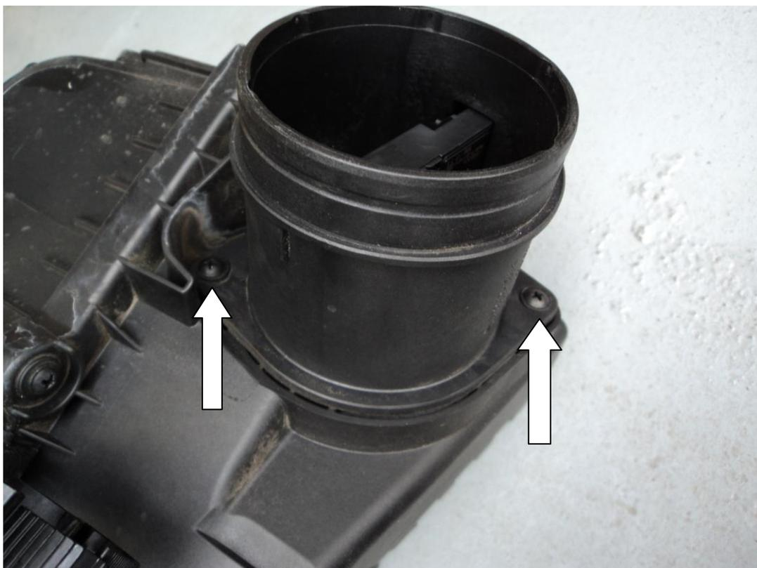
17. Now fit the forge intake to the vehicle using the pictures below for reference.
