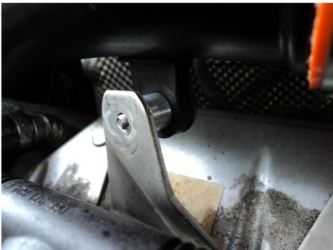
14. Remove the two clips that were previously attached to the standard cold air intake and fit these to the new forge part.
