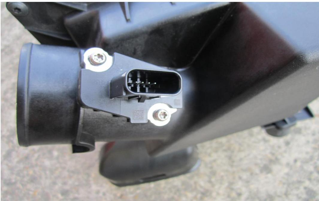
9. Now using the M4 fasteners provided, fit the MAF sensor into the Forge Motorsport MAF housing.
