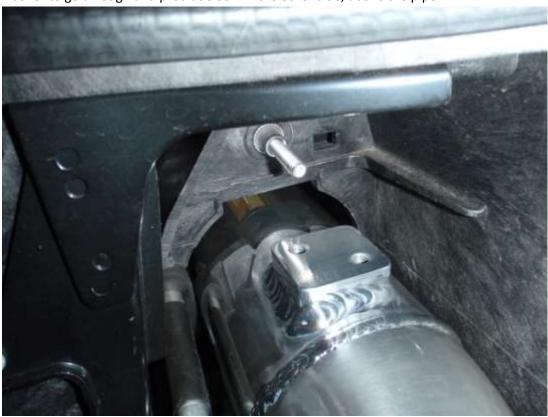
9. Remove the metal bushes from the centre of the rubber grommets supplied, then push the rubber grommets through the holes in the right angled brackets as shown. Once through, push the metal bushes back into position.
