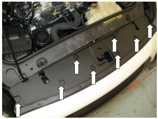
2. First remove the inlet inside the front cowl – undo the single clip and pull the plastic inlet from the filter (shown with bumper removed, not necessary). Also remove the clip and 10mm bolt holding the air guides in and remove them from the car.
