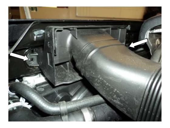
3. Unclip the flexible hose, pull off breather and remove. Unclip the cold air feed by pushing in the sides, Then pull out and remove. Undo the T30 screw and pull up the air filter box until it comes out of the rubber grommets and remove.
