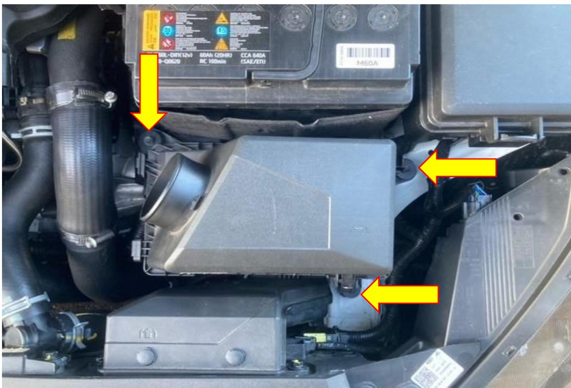
6. Using a 10mm socket and ratchet remove the M6 fastener from the air duct shown in the picture below.
