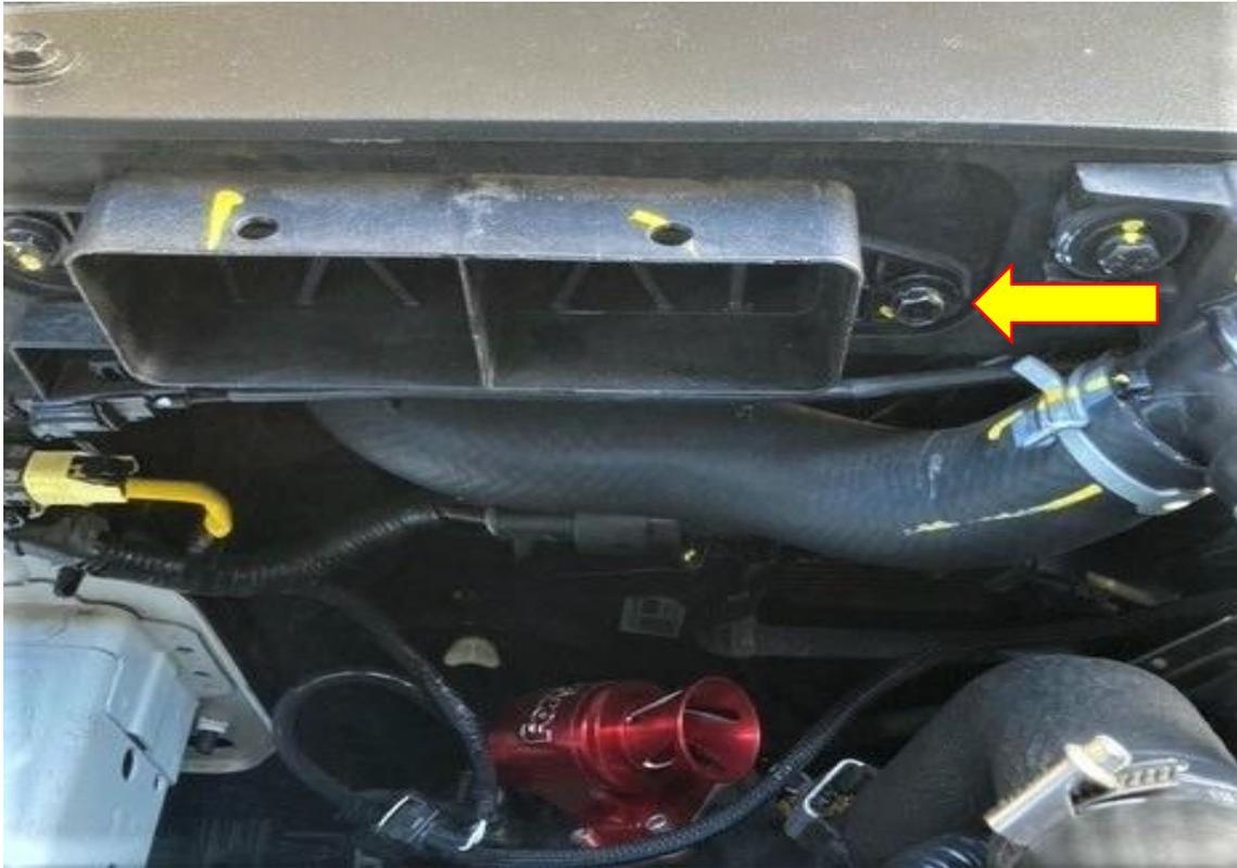
7. Using a 10mm socket and ratchet re-fit one of the M6 fasteners removed from step 5 in the location shown with the arrow.
