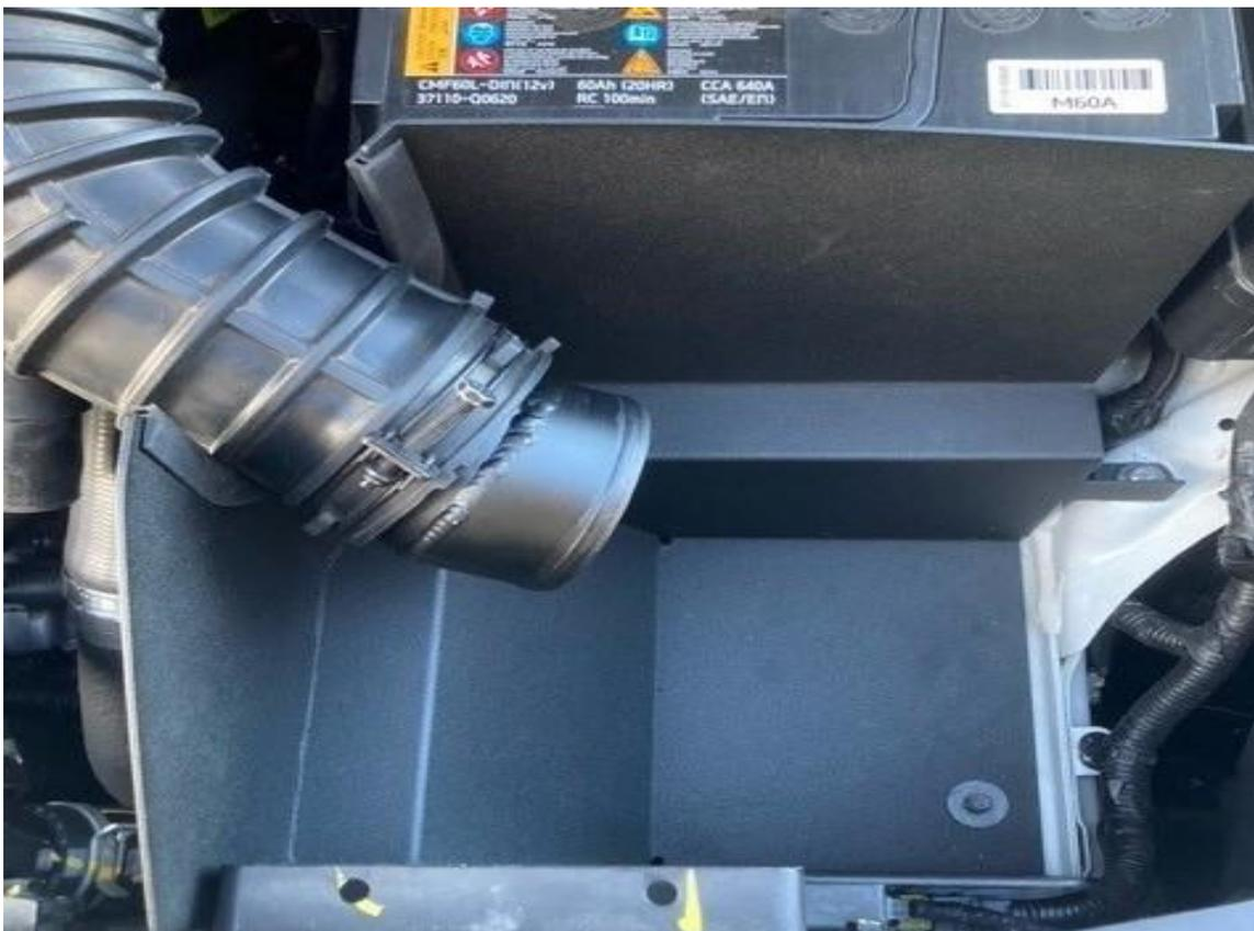
12. Attach the Forge Motorsport air filter to the hose joiner, adjust the orientation of the filter by twisting it round to the desired position. Once happy use a 7 and 10mm socket and ratchet to secure both hose clamps.
