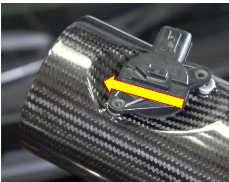
11. Using a 3mm Allen key secure the MAF sensor to the Forge Motorsport airbox lid using the **SUPPLIED M5** fasteners.
