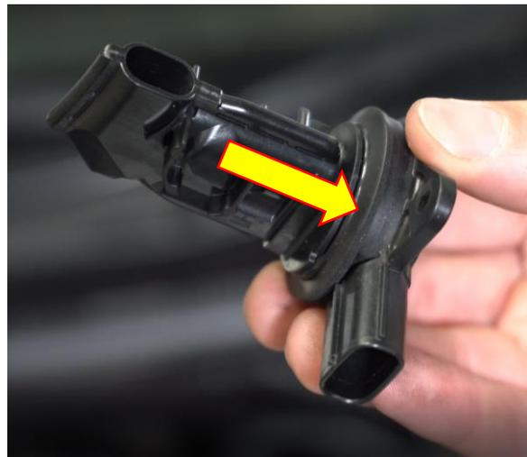
10. Position the MAF sensor into the hole in the airbox as shown in the image below. The arrow will point towards the engine
