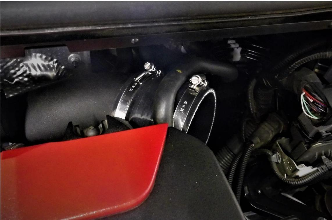
14. Insert the inlet pipe section of the FMINDK43 into the silicone joiner and slide the mounting lugs are located into the bottom part of the OE air box. Tighten the hoses clamps to **2- 2.4nm** secure the silicone coupler, now follow steps 1-4 in reverse order.
