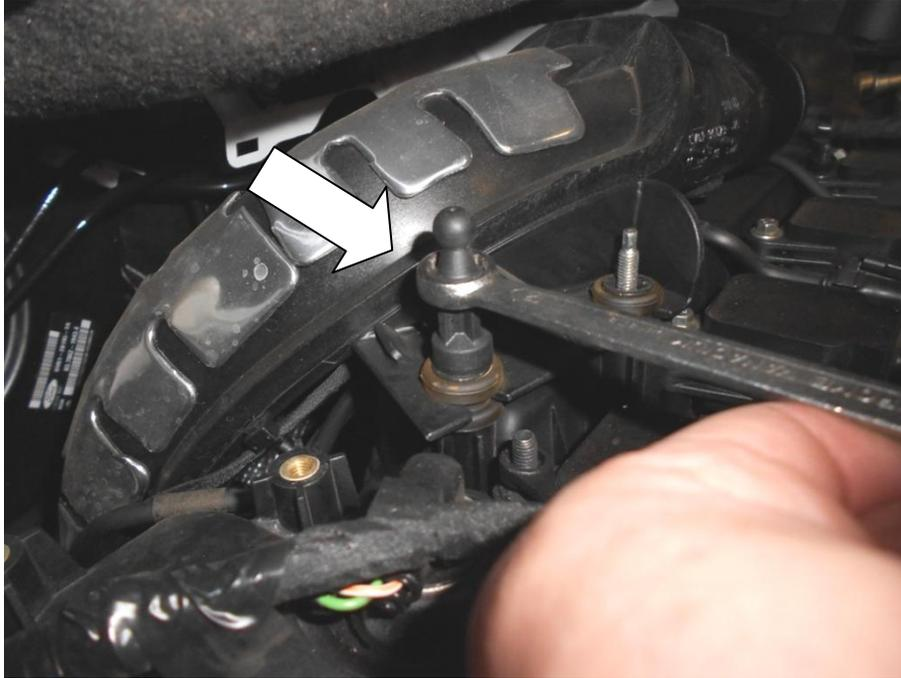
11. Undo the 8mm bolt on the second hard pipe and remove it.
