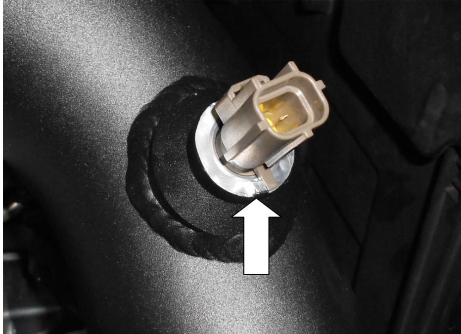
19. Reconnect the wiring to the sensor.
