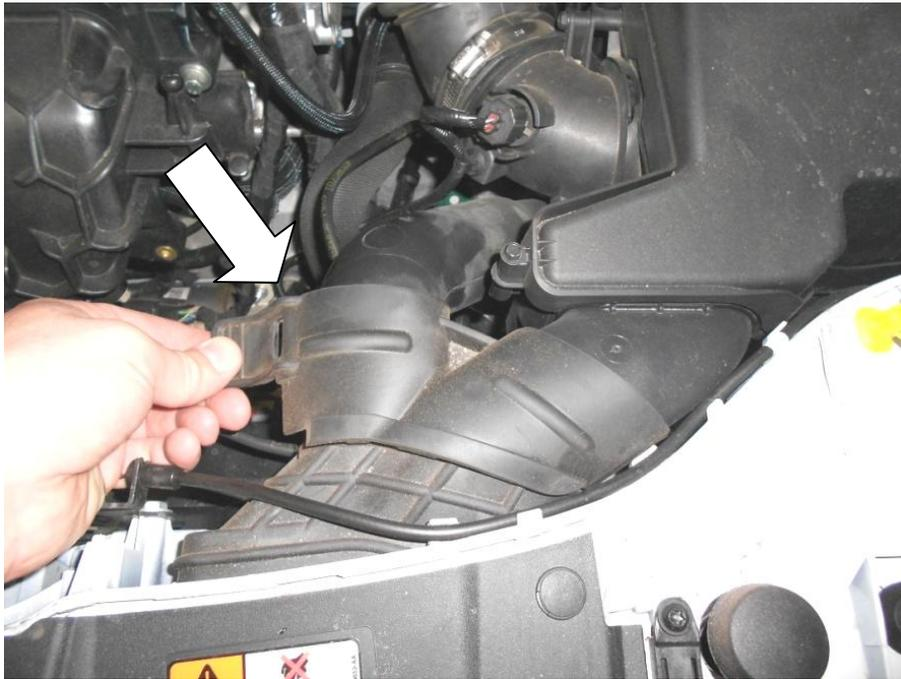
5. Pull the airbox up firmly to remove it.
