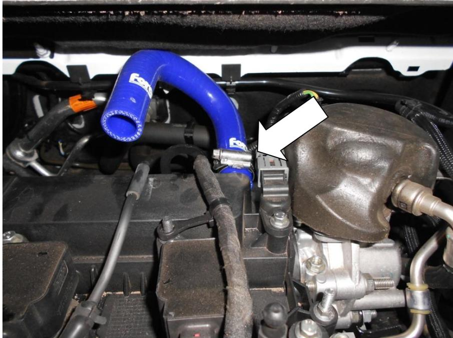
15. Place the 63/76mm silicone reducer on the turbo inlet and secure with a suitable hose clamp.
