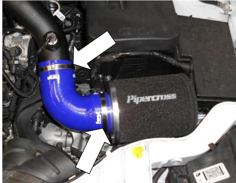
22. In the open end fit the Pipercross Filter and secure with the last hose clamp.
