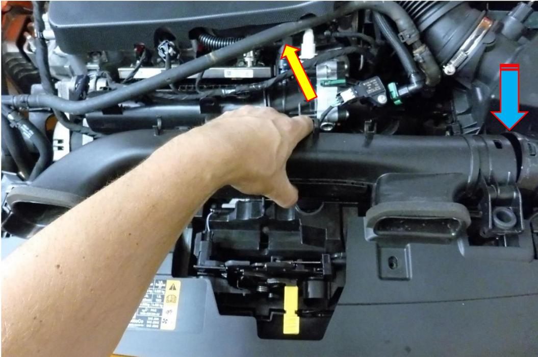
3. Twist the MAF sensor anti clockwise and remove it from the airbox, there is enough length in the cable to place it on the battery for now. Using a 7mm socket and ratchet loosen the hose clamp enough so the hose can be removed. Pull the airbox sharply in an upwards motion and remove from engine bay.
