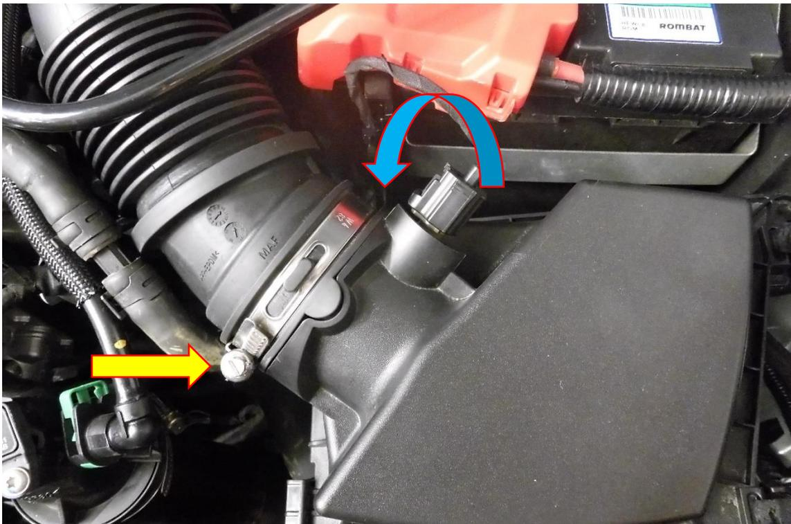
4. Fit the Forge Motorsport air filter tray into the engine bay, make sure both mounting pegs on the tray locate into the OE rubber grommets.
