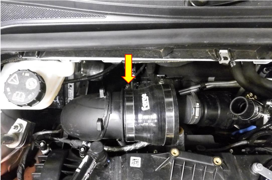
12. Fit the Forge alloy intake to the silicone reducer and silicone diverter valve hose. Use the hose clamps to secure it. Re attach the oil breather pipe and tighten the cam cover fastener to the mounting bracket on the intake pipe.
