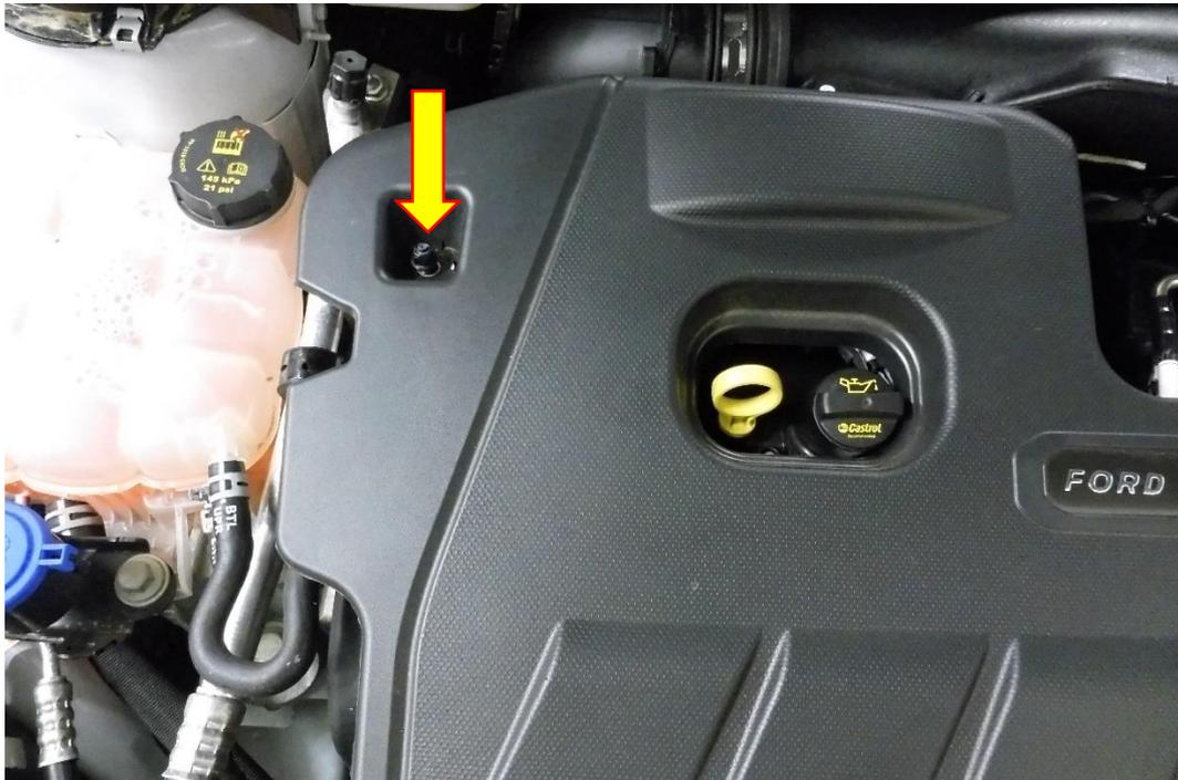
2. Using an 8mm spanner or socket and ratchet remove 2X 8mm fasteners attaching the intake pipe to the engine. Using hose removal tool or long nose pliers release the diverter valve pipe attached to the back of the intake pipe, to remove the oil breather simply pinch the retaining clips and pull the pipe away from the intake pipe.
