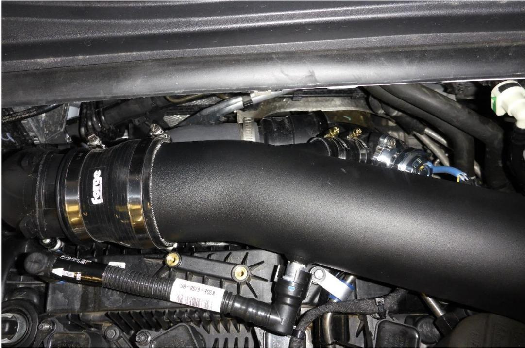
13. Re fit the MAF to the MAF boss on the intake pipe.
