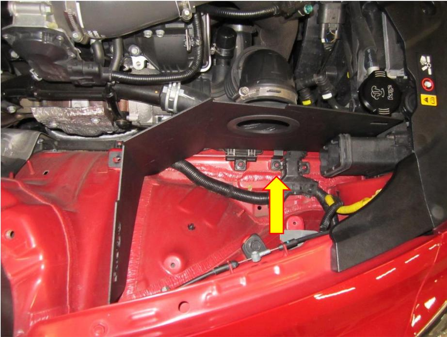
5. The nearside is very similar to the offside, as before place the heat shield in the engine bay and line up the brackets as shown in the picture below. Re fit one of the fasteners at the front of the heat shield to hold it place.
