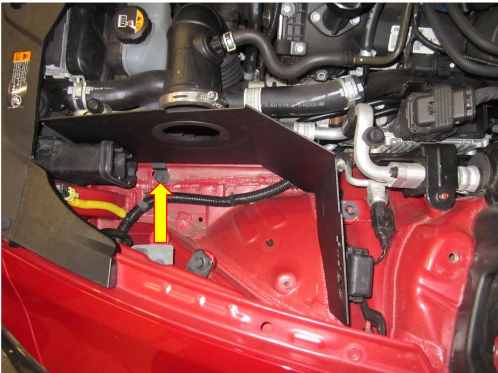
6. You will now be able to install the filter by angling the heat shield backwards and pushing the alloy filter neck through the hole in the heat shield. Insert the alloy end of the filter into the intake hose and tighten the hose clamp while pushing down on the intake hose at the same time.
