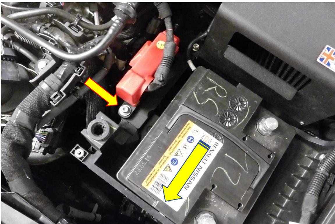
25. Supplied in the FMINDK31 kit is a silicone sleeve, wrap this around the non-insulated part of the POSITIVE battery terminal. Use the supplied cable ties to secure it in place.
