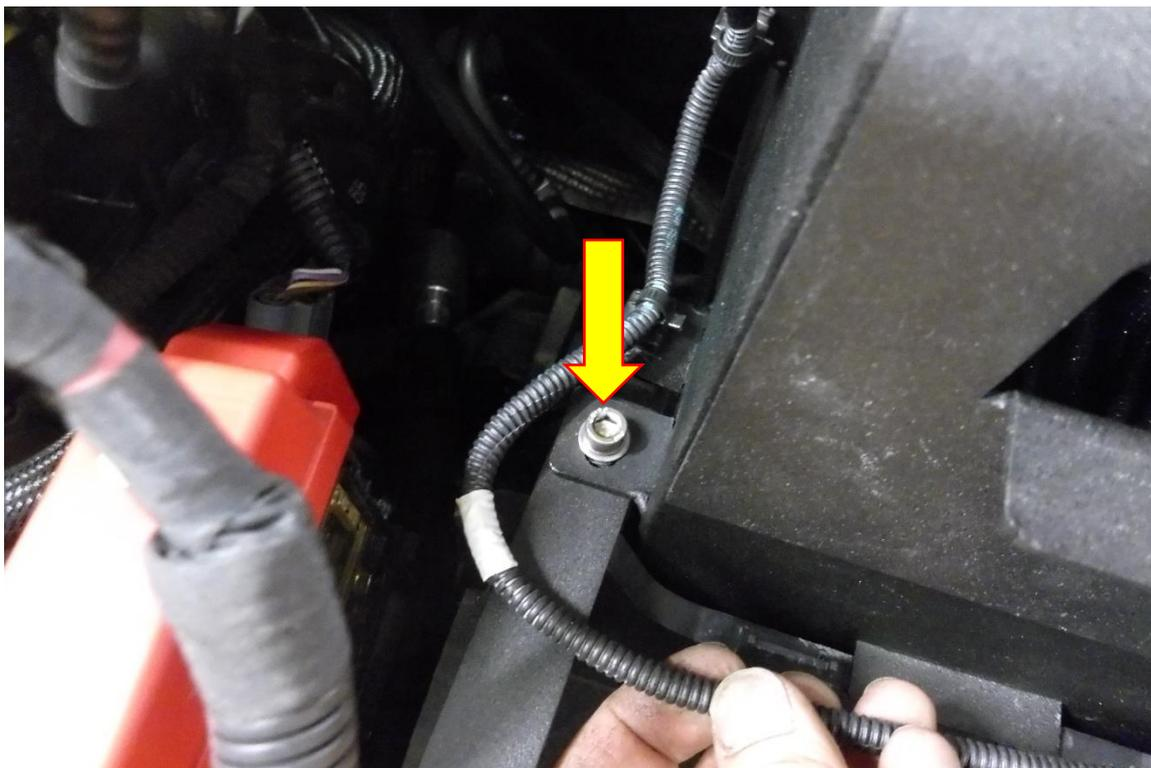
24. Re install the battery and slide it as far as possible to the front of the vehicle and secure it down, re attach the battery fuse box while clamping down the mounting bracket. Re install the battery cover.
