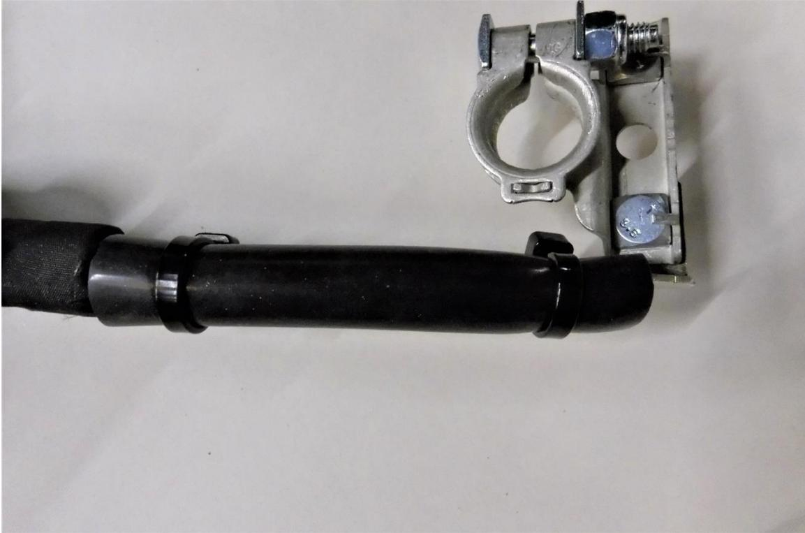
26. Fit the POSITIVE battery terminal as shown in the picture below.
