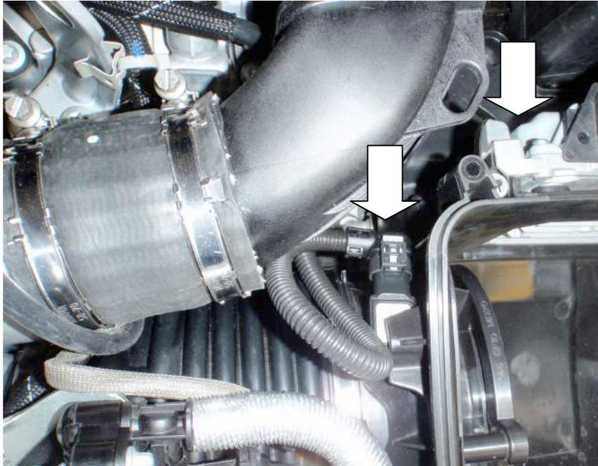
4. Using a T25 Torx driver remove the 3x screws and remove the standard airfilter adapter from the airbox.
