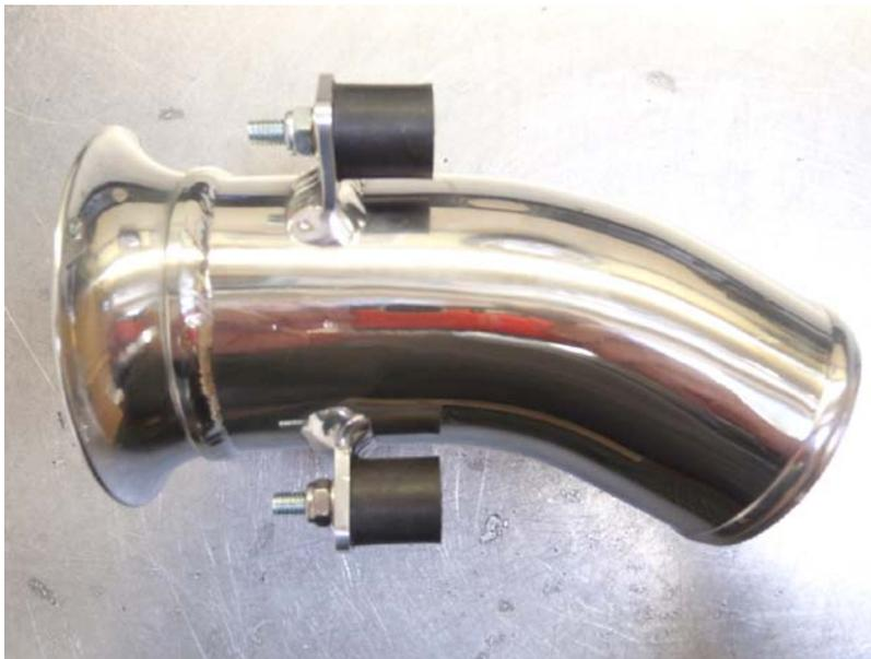
12. Bolt on cotton reel rubber mounts with two M6 nuts and washers to inlet pipe.
