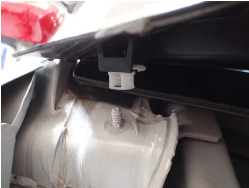
8. Now lift the panel upwards and in the far corners you will see a white clip. Pull upwards to remove.
