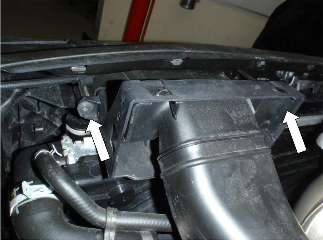
4. Undo the T30 torx that is holding the air box down, pull the air box upwards holding the 2 leading edges to release it from its rubber mounts removing it from the car.
