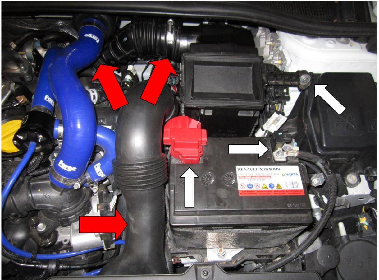
2. Then remove the cold air inlet pipe and undo the hose clamps on the inlet hose with your hose clamp driver. These are arrowed red in the picture above.
