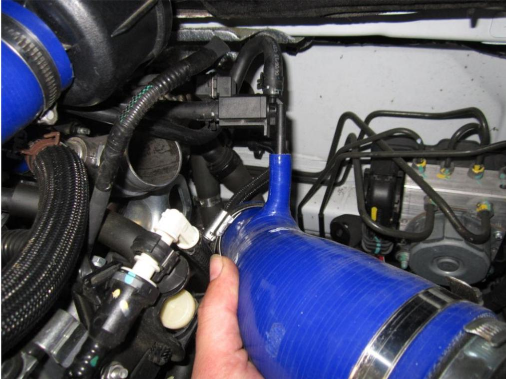
7. Once your new performance airfilter is in position, tighten the hose clamp at the turbo inlet end of the hose.
