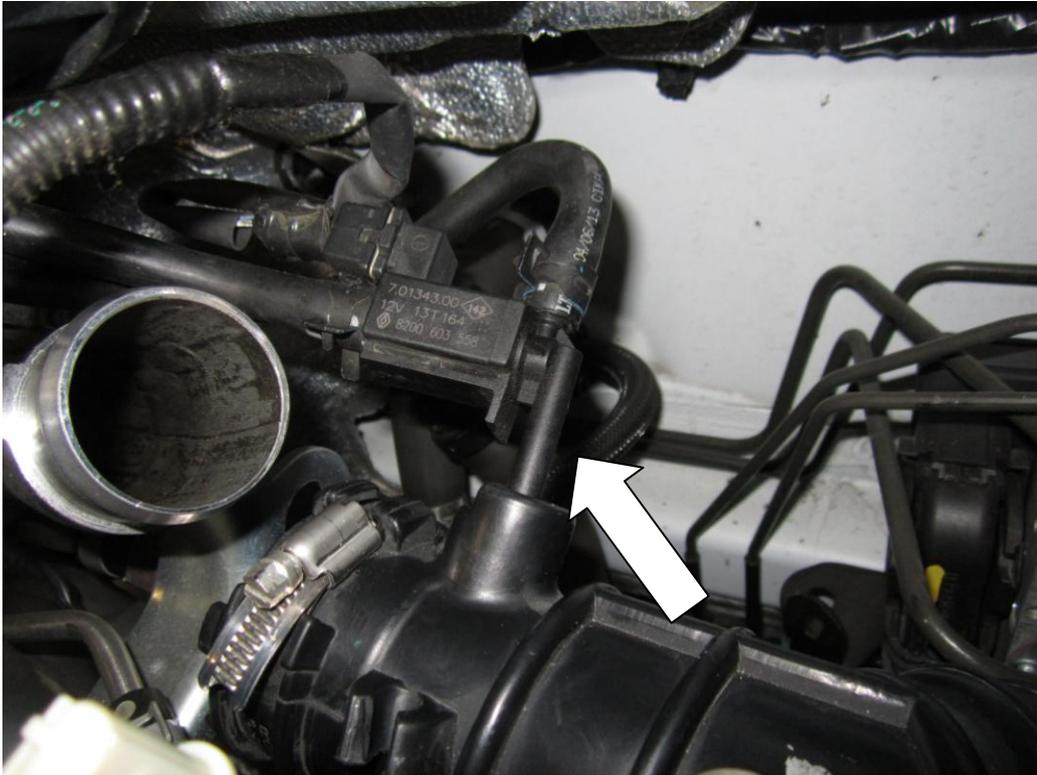
5. Now assemble the forge performance airfilter into the new forge motorsport induction hose leaving the hose clamp on the smaller end loose.
