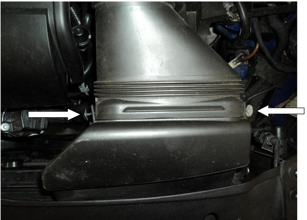
5. Undo the two T25 torx (one each side) holding the cold air scoop to the slam panel.
