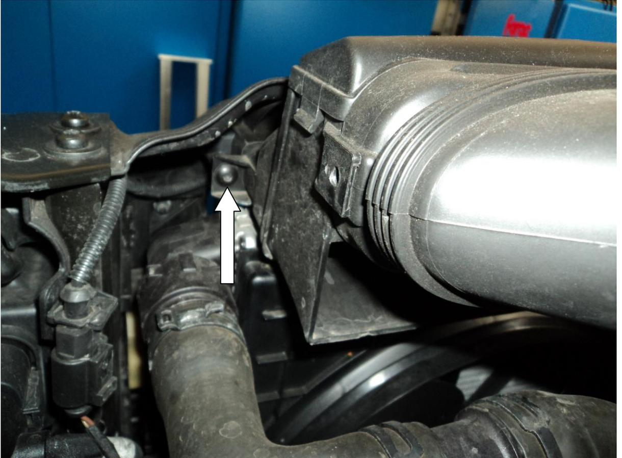
6. Now remove the engine cover by pulling up on the 4 points shown below.
