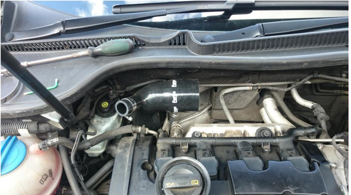
8. Using a 10mm spanner, remove the two 10mm nuts on the underside of the engine cover mounting points. Once these are removed, use a 24mm socket/spanner to undo the two black plastic engine cover locaters.
