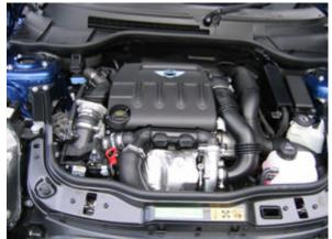
installation as the system will be pressurised if the temperature has risen. Great care is need in the removal of the tank cap as pressure may be released.
