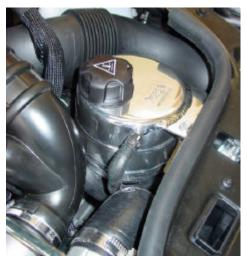
cap opening. The cap from the original tank is re-used and secured.
