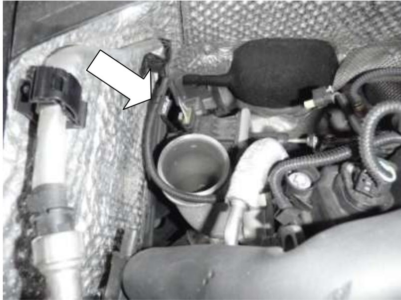
12. Carefully pull the intake pipe upwards and pull the coupler off the turbo inlet.
