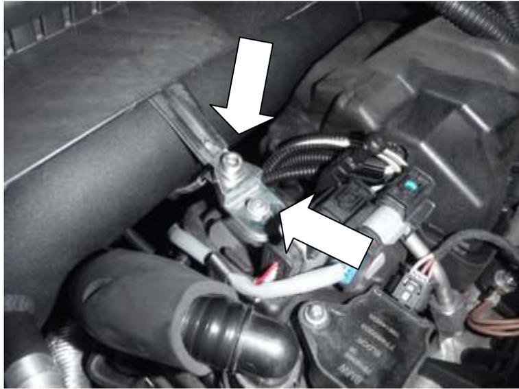
24. Refit the standard air box and intake scoop.
