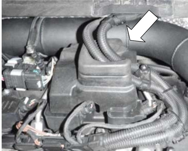
16. Carefully remove the intake pipe. Check that while the pipe is being removed it has not become snagged on any of the wiring behind the engine.
