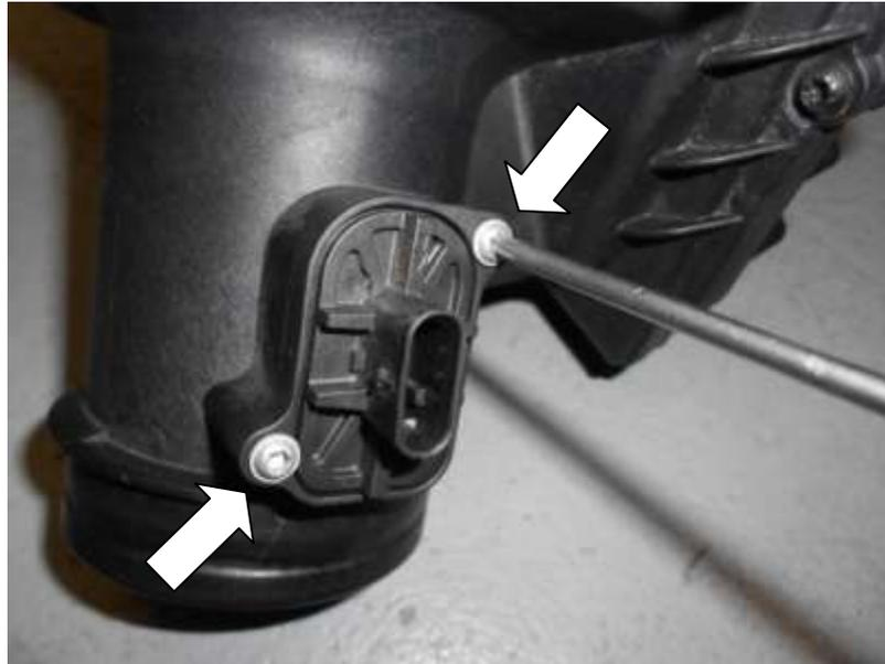
28. Fit the MAF sensor to your Forge Alloy induction pipe and secure using the 2x M3x12mm Allen cap bolts. The Arrow on the sensor pointing towards the engine.
