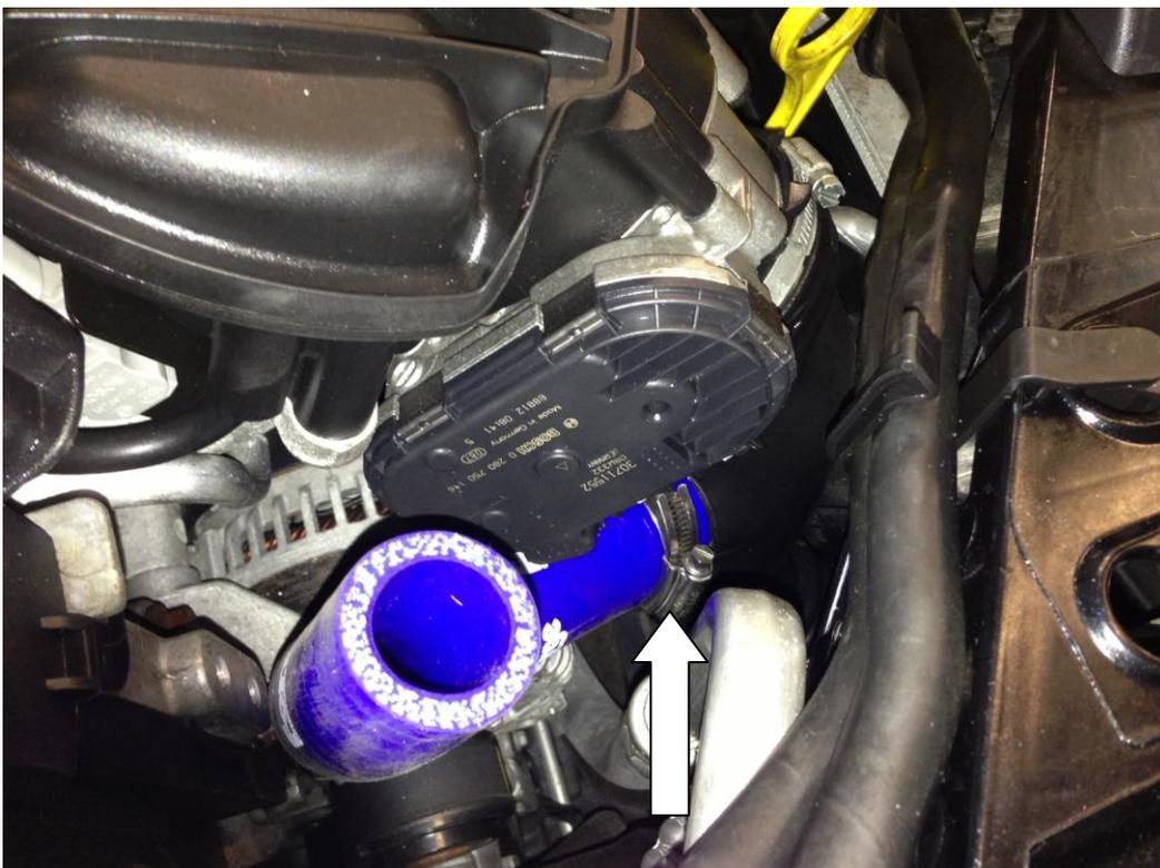
8. Place the smaller hose clamp over the hose and place the new valve into the other end of the silicone hose. Again using a hose clamp driver tighten the hose clamp around the valve.
