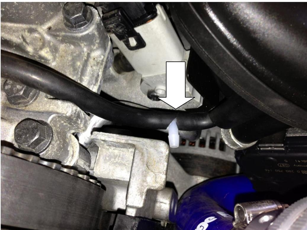
10. Last step is to simply place the vacuum hose provided over the plastic "T" piece and then to the vacuum nipple on the top of the valve. You may wish to trim the vacuum hose to desired length. Now refit the cambelt cover and test drive the vehicle.
