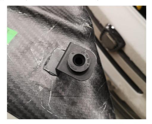
8. Now that you have all three rubber grommets attached to FMEC4, take the supplied red grease, and smear a small amount onto the centre of each of the three grommets similar to as shown below.
