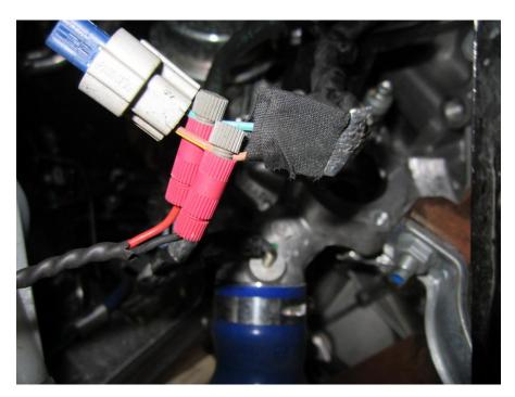
13. Then attach the forge wiring loom to the posi locks
