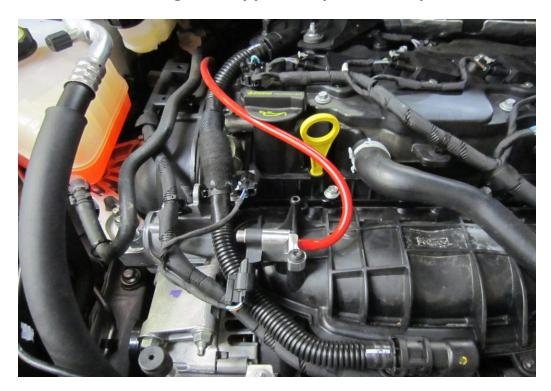
11. The vaccum line that is red (FOR ILLUSTRATION PURPOSES ONLY) needs to be attached to the solenoid. Run this down the back of the engine using the zip locks provided keeping it away from any hot sources or moving parts as pictured.
