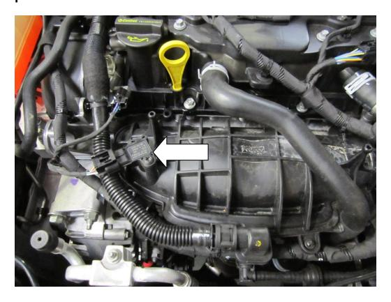
10. Fit the boost take off block supplied using the T25 torx screw. Fit the boost sensor using the supplied cap screw as pictured below.
