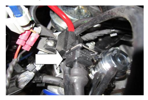
15. BEFORE STARTING THE VEHICLE DOUBLE CHECK THE CONFIGURATION ON THE WIRING LOOM AND VACCUM LINES TO THE SOLENOID.
