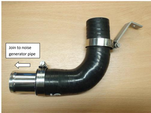
9. Fit the valve to the end of the pipe and tighten the jubilee clip whilst positioning the bracket over the hole in the firewall. Use the bolt and plain washer on the top of the bracket, and penny washer and nyloc nut on the bottom to secure the bracket. Connect the vacuum hose to the top of the valve and the installation is complete!
