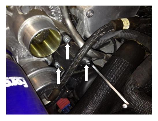
5. Remove your Forge valve from the box and insert the o-rings supplied into the bottom face of the valve, then bolt the valve to the turbo using the bolts supplied. Note the valve will only fit one way round, meaning the vacuum port on the base of the valve points DOWN (the port on the top of the valve can be pointed in any direction).
