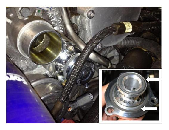
6. Locate the vacuum pump on the end of the head (just behind the valve), and pull off the vaccum pipe shown below. Then cut a short length (50mm) of the silicon vaccum hose supplied and push it on to the outlet on the pump. Use the tee-piece provided to join the new silicon hose to the old vaccum hose, and point the tee piece forwards in the engine bay.
