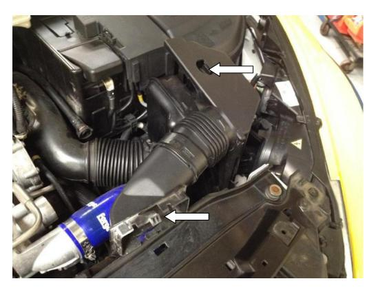
3. Remove the intake resonator by pushing the clip shown so that it releases from the bracket on the chassis leg, then lifting the resonator vertically upwards out of the bracket. Once this is free, you can pull the cold air feed pipe from the bottom of the filter – its a simple push fit – and remove the resonator and connecting hoses from the car in one complete unit.
