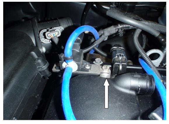
8. Remove the vacuum hose situated in the side of the head to the right of the valve.
