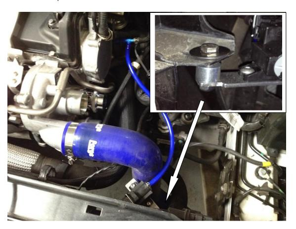
9. Connect a vacuum hose to the LOWER port on the dump valve. You may find it easier to unscrew and remove the top of the valve to do this. If you do, make sure you catch the spring as you unscrew the top. Route this vaccum hose to the REAR METAL port on the solenoid, cut the hose to length and fit.
