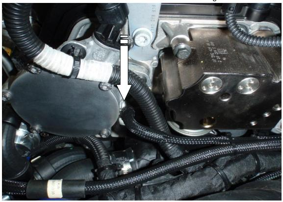
9. Now using the silicon hose and the 5mm T piece provided fit the silicon pipe as shown using the diagrams below.
