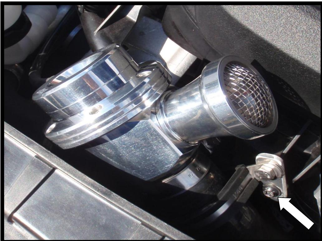
7. Remove the inlet pipe from the filter
