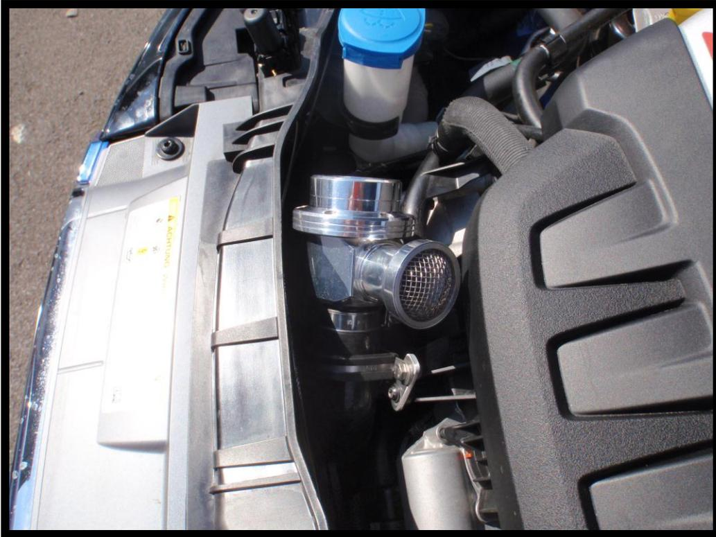
6. Fit the dump valve with hose clip and P-clip using the small bracket and bolt supplied in the kit. Attach to the inlet manifold and tighten using the screw previously removed.
