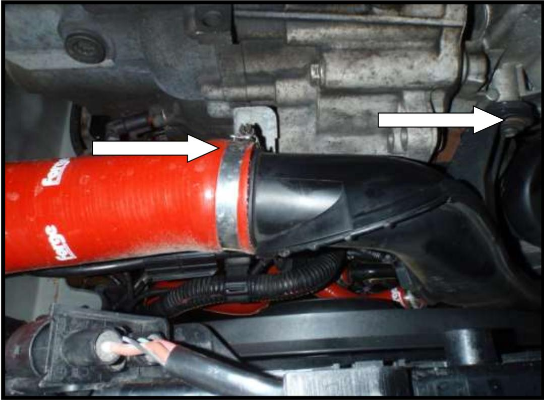
6. Remove the MAP sensor and install the boost take off block using the long screws supplied. Please note the cork gasket is between the pipe and the block, the boost take off is also closest to the plastic pipe as shown below.
