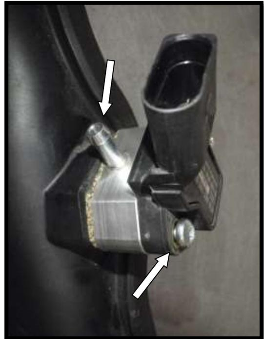
7. Install the new plastic turbo pipe in reverse to removal.
