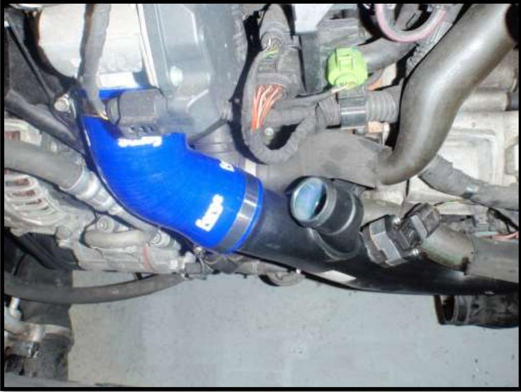
8. Install the silicone hose and BOV with the clips supplied in kit.
