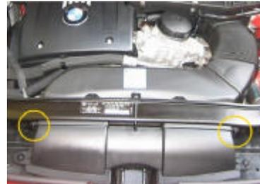
2.) Next, disconnect the rear section of the intake scoop that leads into the air box (circled at right). To disconnect this, simply squeeze on the top and bottom of the snorkel until it is free of the tabs on the sides. Then, simply pull outward gently. Now that this is free, you can remove the entire intake scoop from the car.
