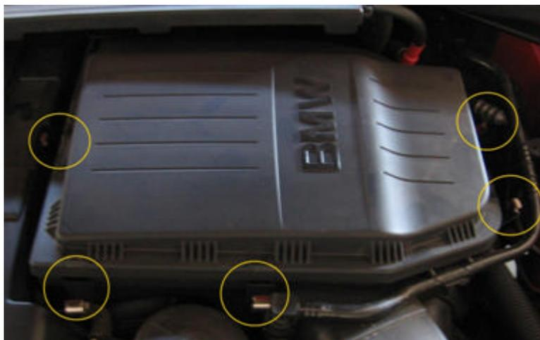
4.) Disconnect the small hose at the front of the air box. To remove this hose (circled below) simply squeeze the sides of the plastic ring connector and pull up. Then pull the hose away from the air box where it is held in place at the corner.
