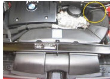
3.) With the intake scoop removed, you will next remove the air box cover. To do this, simply unhook all the metal clasps holding it on. There are five clasps (circled below) located around the outer edge of the cover. You can then lift the cover off, and remove the air filter from the air box.
