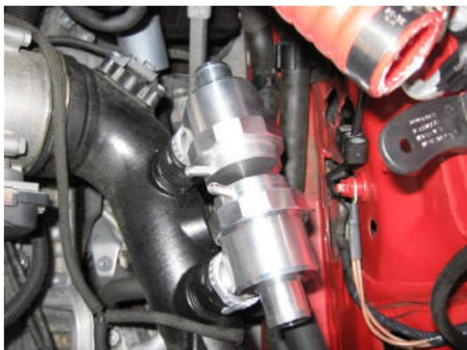
11.) Next, you will install the included silicone hoses. You will notice the two hoses are slightly different lengths. One is 13" long and the other is 16" long. The longer hose (16") will install from the rear most valve to the port at the back of the engine bay. The shorter hose (13") will install from the front most valve to the port at the front of the engine bay. We will start with the front hose (the shorter of the two).
