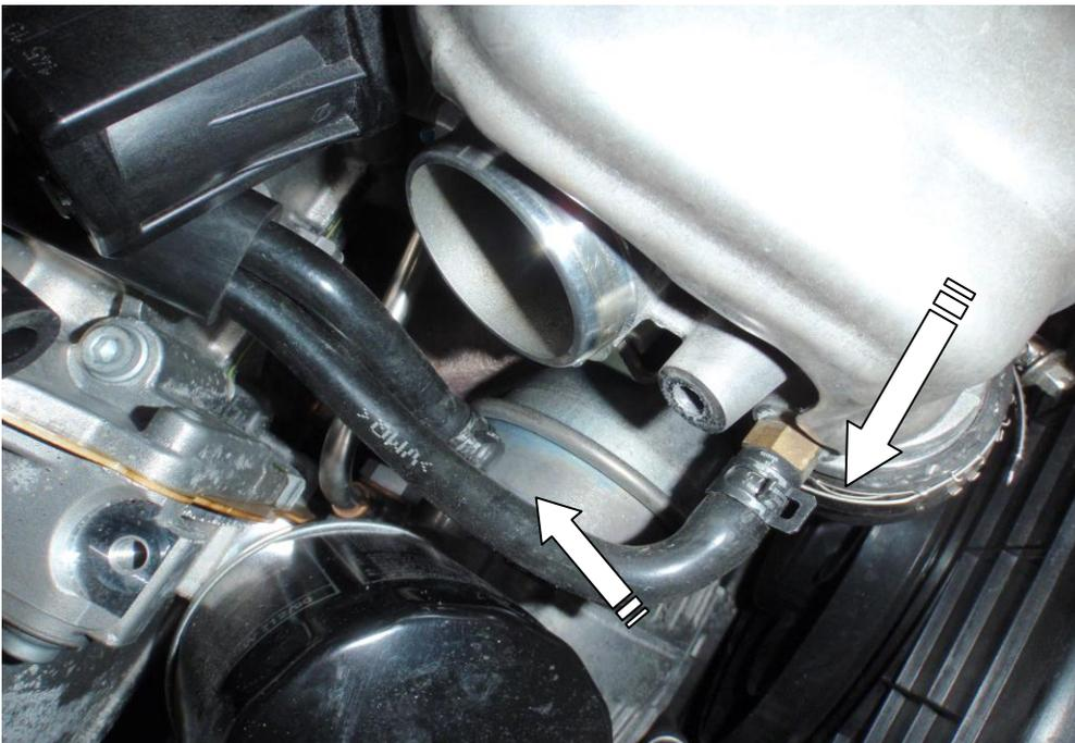
5. Using the T30 torx, undo both screws holding the standard valve in place.
