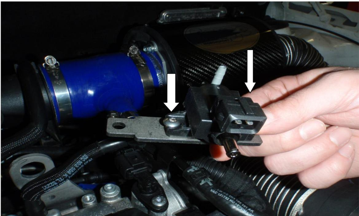
15. Locate the hole in the engine bracket. Place the 5mm Allen bolt through the bracket then through the hole, once that is done screw the m5 nyloc nut ( that is provided) onto the bolt and tighten using a 3mm Allen key and 8mm spanner, as seen in the 2 pictures below making sure the orientation is correct.
