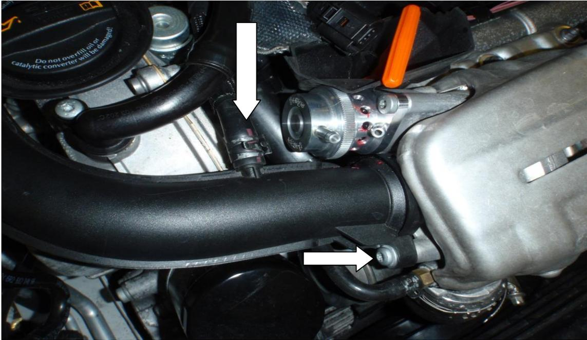
10. Now remove the pipe coming from the purge control solenoid by simply pulling apart. Once the pipe has been disconnected pull the purge valve out of its plastic bracket by pushing the valve towards the back of the car (This will make it easier to get to the vacuum take off at the back of the engine).
