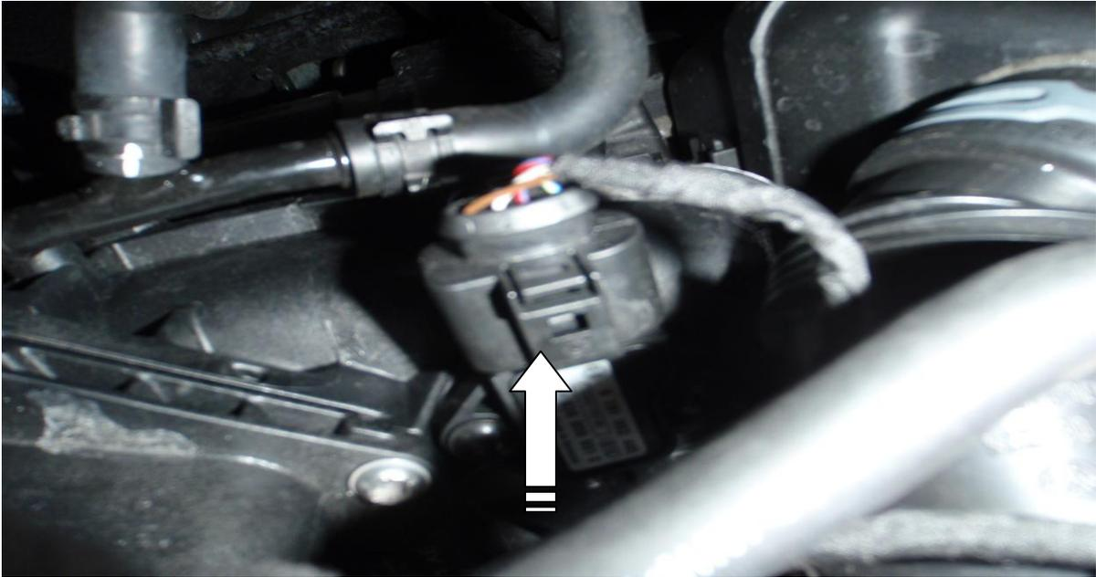
12. Now using the sensor push it into the forge vacuum takeoff block as shown in the picture below making sure to get the orientation correct. While you're at this stage it will be easier to push the silicon vacuum pipe onto the vacuum take off outlet port as seen below.
