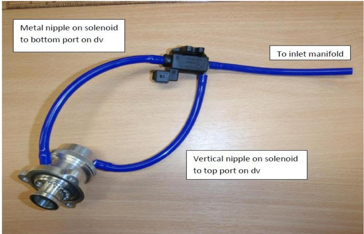
18. Using the cable ties provided at your own discretion, tidy and support the vacuum pipe and new wiring loom.
