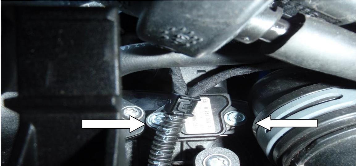
14. Using the bracket, solenoid and the two 3mm Allen key bolts provided, place the solenoid onto the bracket and screw down using the two 3mm Allen key bolts making sure the orientation is correct as seen in the picture below.
