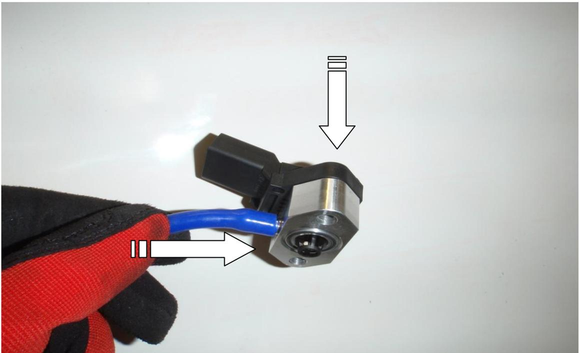
13. Now replace the sensor along with the vacuum take off block back into the inlet manifold where which the sensor came from originally using the two 8mm self tapping screws provided and push the plug back onto the sensor making sure the “o” ring on the bottom of the vacuum take off plate is seated correctly and does not fall out while installing. (As seen in the picture above).
