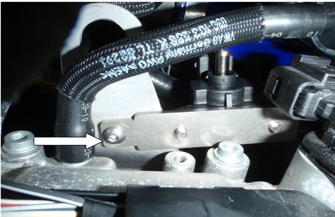
16. Now that the bracket and solenoid is in place, plug the wiring loom that is provided into the top of the solenoid, and the other end into the standard valve plug.
