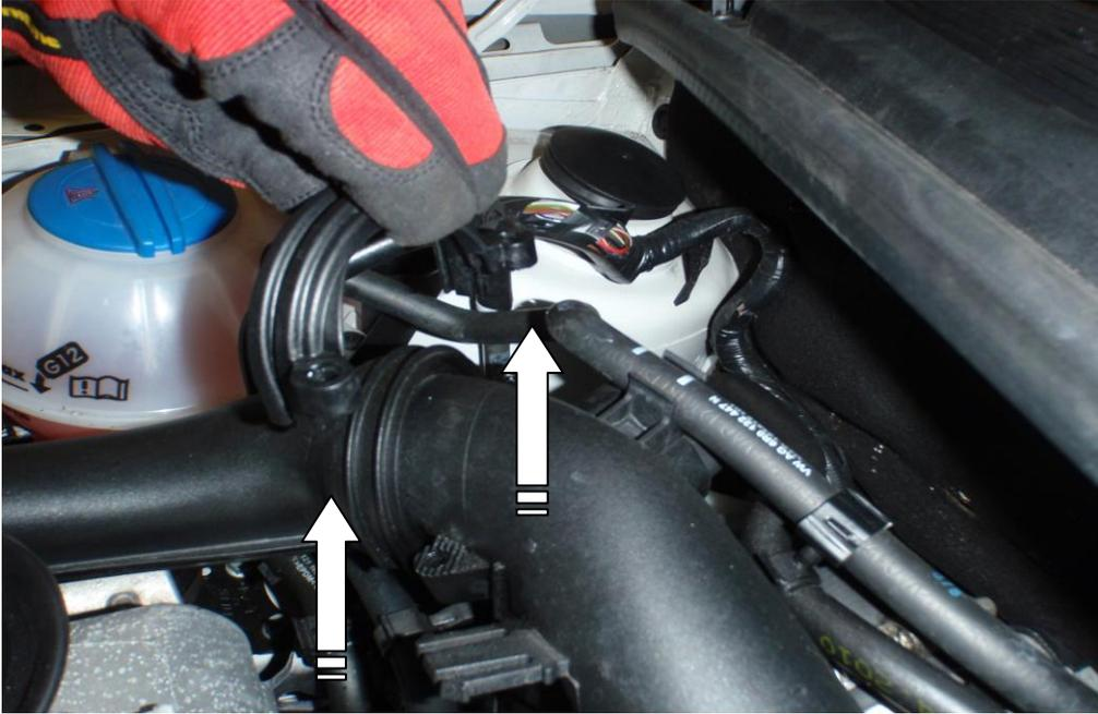
4. Using a pair of pliers squeeze the 2 hose clamps that are on the rubber hoses to move them out the way enough to remove both pipes.
