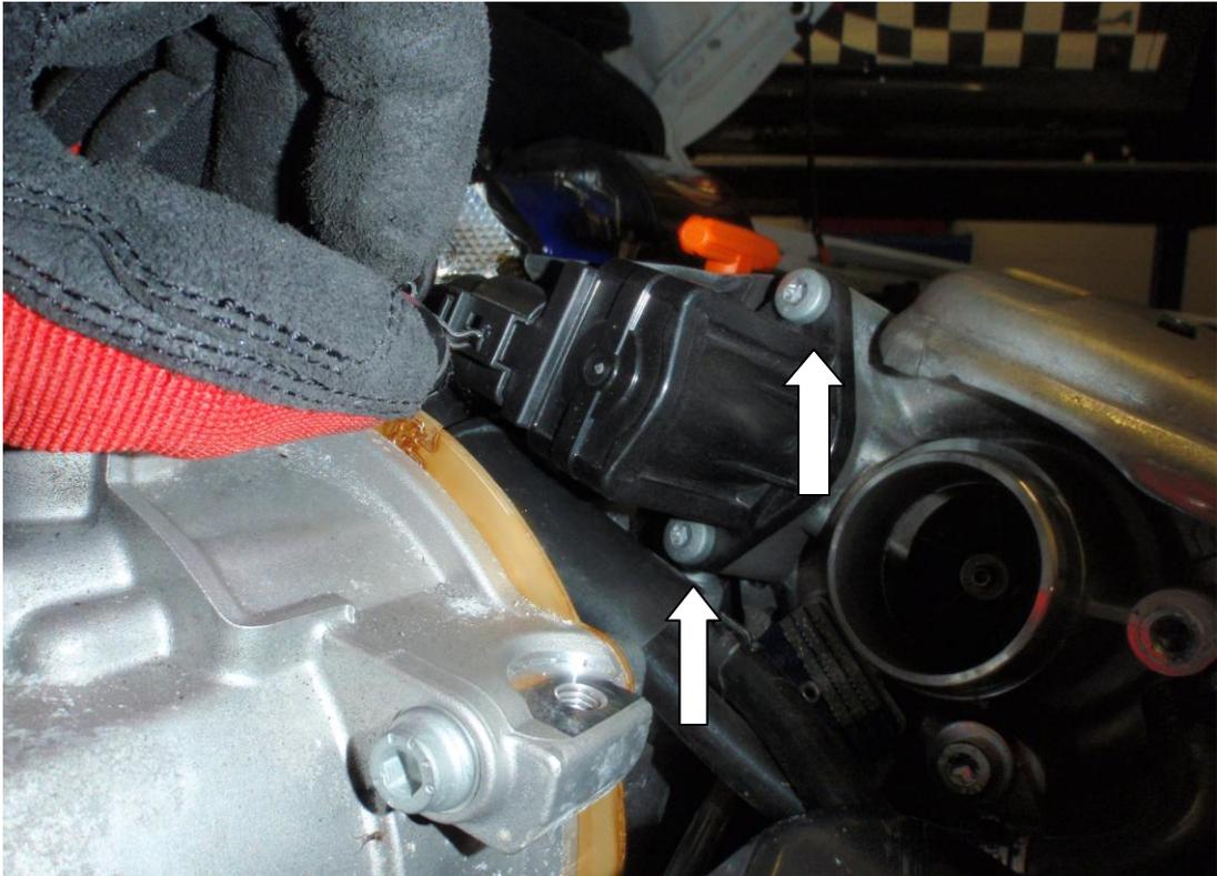
6. Undo the plug attached to the standard valve by pressing the tab and pulling the connector away from the valve.
