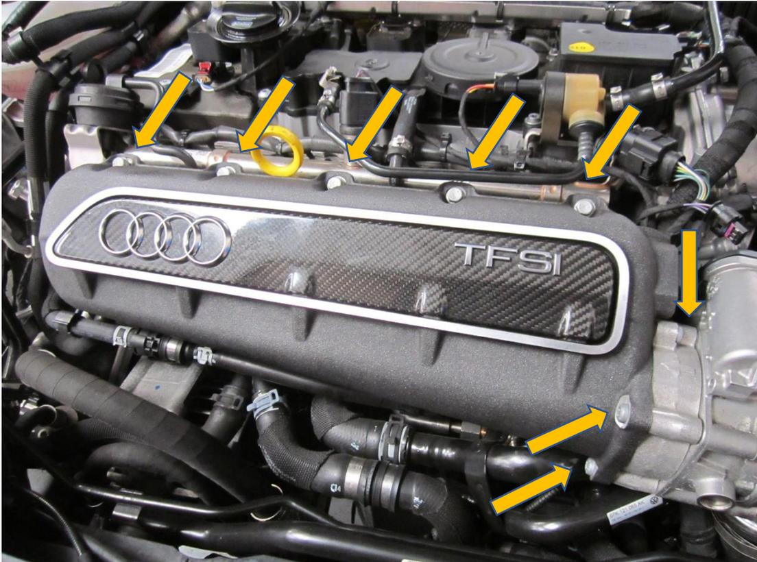
4. Split the inlet manifold in order to remove the last T30 fastener that holds the throttle body to the inlet manifold.
