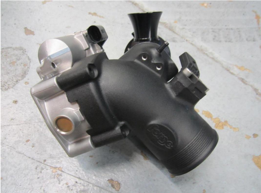
6. Attach the MAP sensor with the m6 x 16mm bolts supplied along with the plastic engine cover bracket.
