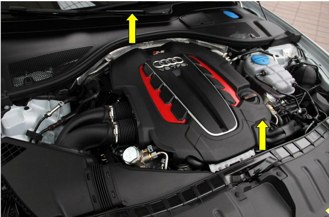
2. Using a flat bladed screwdriver pry off the clip that holds the water pipe from the charge cooler to the dump valve housing, then undo the 6 T30 fasteners arrowed red.
