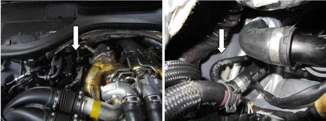
10. You must now cut the vacuum pipe in picture two and insert a brass T-piece with the silicon vacuum pipe connected.
