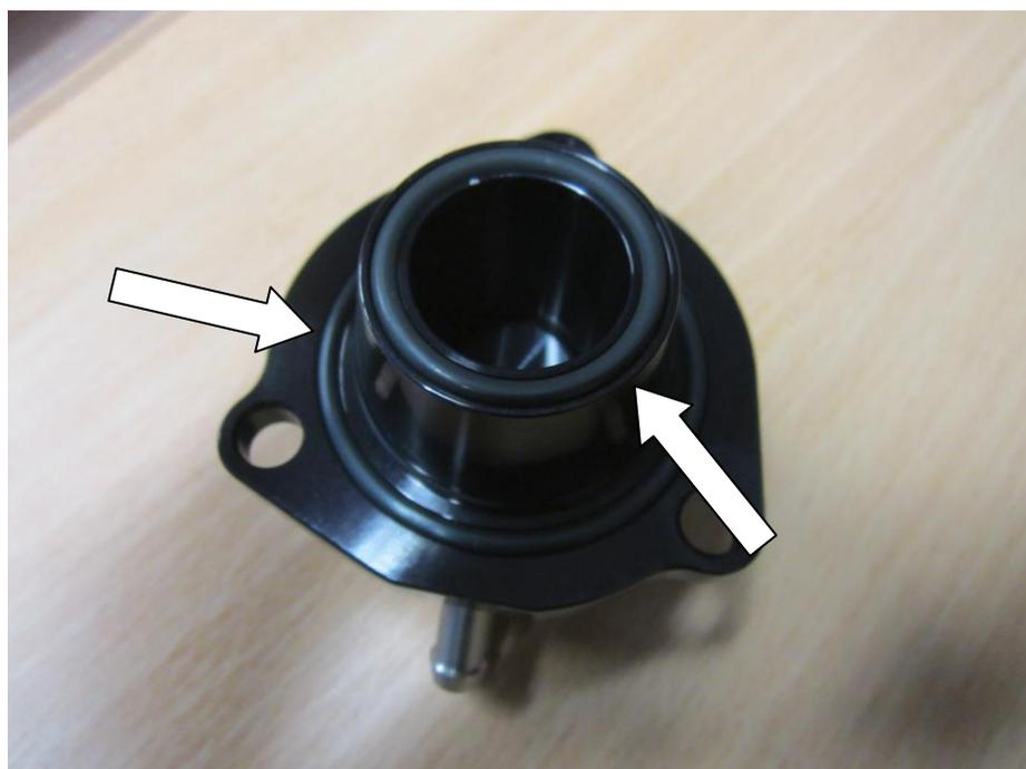
6. You can now fasten the Forge Motorsport valves to the housings again using your T30 Torx driver. Please note the orientation of the valve.
