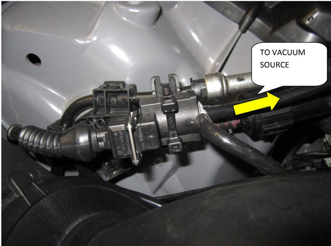
12. Now your valves are in situ, using two suitable lengths of silicon vacuum tubing, connect both the lower nipple and upper nipple of each valve together as pictured below.
