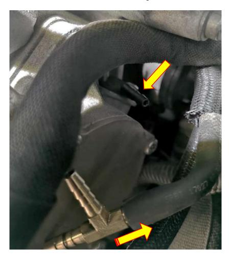
15. Cut a section of supplied vac line to join an opening of the T piece to the OEM vac pipe.
