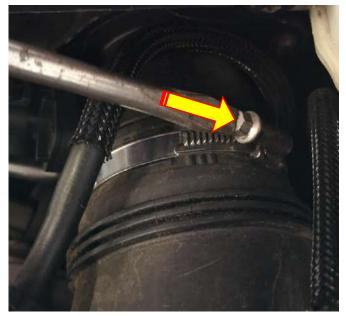
7. Pinching your fingers on the flat areas of the clips will remove the two breathers from the right-hand side of the inlet pipe
