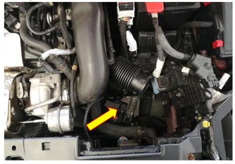
5. To remove the inlet pipe to the turbo we need to undo it from the points labelled below, as shown in the following steps
