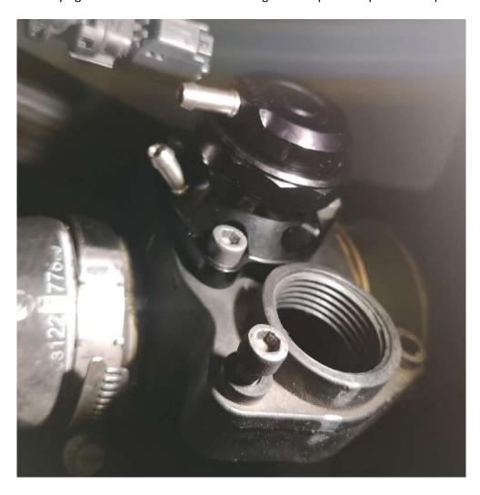
23. Using a 3mm allen key tighten the two bolts to secure the solenoid to the plate in this orientation.
