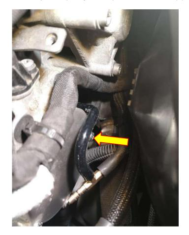
16. Cut a long section of supplied vac line and connect one side to the T piece to seal it off. This vac line will be running to the valve so leave this long for now as you can cut it back in a later step. Use the supplied cable ties to secure all 4 vac line points (one to OEM vac pipe at vac pump, and one for each vac line on the T piece)
