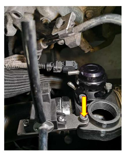
26. Using a safety blade cut the vac lines to length according to the images below. Routing the vac lines is **EXTREMELY IMPORTANT.** Please use the diagram and images below to help route the vac lines to the correct ports.
