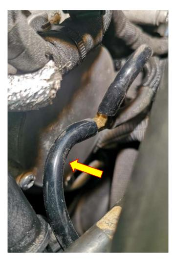
17. By using your hand you can unscrew the resonator pipe to give more access room to the valve.
