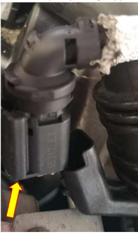
**11**. Using a hose clamp removal tool or long nose pliers loosen the hose clamp from the base of the plastic, over the ribbed section and place it on the tube as shown in the image below
