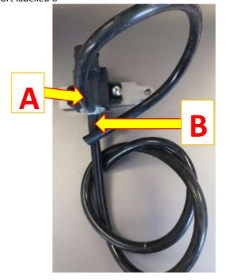
25. With a 5mm allen key undo the OEM bolt shown place the solenoid and bracket into position and tighten the bolt back up allowing it to still move with relative freedom. This is so that you can shift the solenoid around when fitting the vac lines
