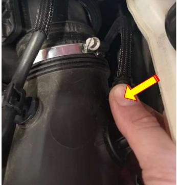
8. Push the green clips into the vac pipe that is situated on top of the vac pump to disconnect it
