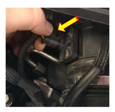
10. Take your flathead screwdriver and gently insert it into the bottom of the sensor as shown by the arrow below, that will disconnect the clip and you can gently pull it from the top to disconnect it.
