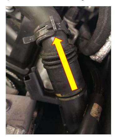
12. The inlet pipe should now be free for you to pull it to the right-hand side, leaving it in the position as shown below which will allow us access to a vac pipe.
