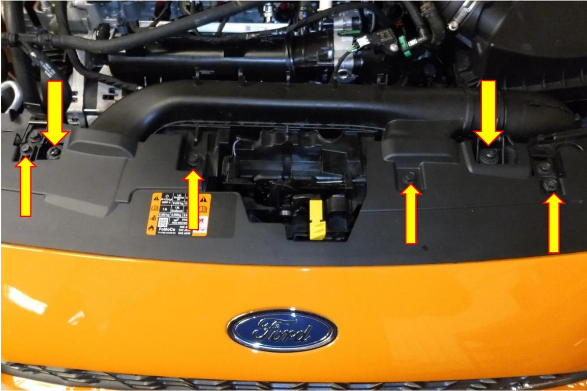
2. Push in both retaining tabs attaching the intake ducting to the airbox, this will then allow you to remove the intake ducting from the vehicle.
