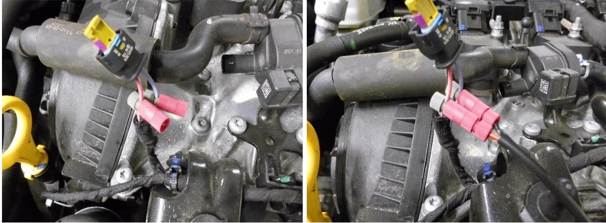
15. Cable tie both silicone hoses and the wiring loom to the valve with the vehicles wiring harness running down the side of the engine.
