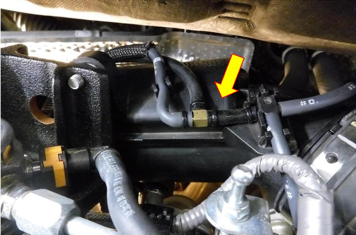
5. Attach the vacuum hose to the solenoid to the spout with the arrow.
