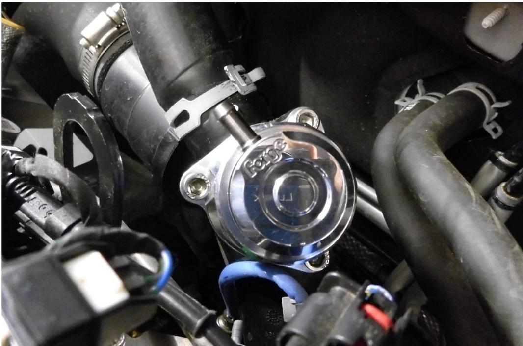
7. Take the solenoid, bracket and the X2 M4 fasteners and assemble as shown in the picture below using a 2.5mm Allen key to tighten the fasteners. Now attach the solenoid to the back of the engine using the supplied M6x10 Allen cap head bolt and spring washer.
