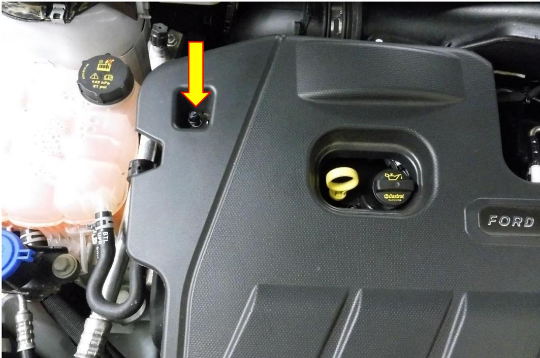
2. Remove X2 8mm fasteners attaching the intake pipe to the engine using an 8mm spanner or socket and ratchet. Remove both breather hoses, the breather closest to the front of the vehicle simply unclips and the hose at the rear will need long nose pliers or a hose clamp removal tool to release it.
